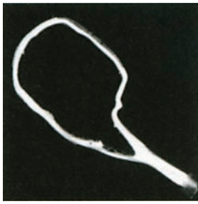
FIGURE 9. CT slice of Roman bronze bull, first century B.C.E. to first century C.E., showing extent and specific depth of plaster restorations.
