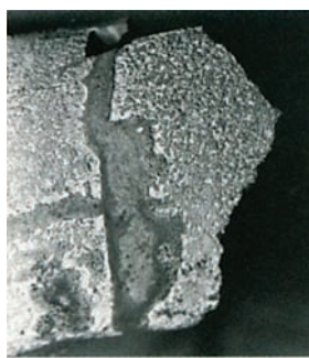
FIGURE 9. Detail of the severely corroded right wrist, Neptune Fountain. Dark material is lead-tin solder.
