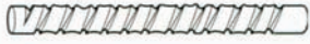
FIGURE 5. Diagram of spiral-beaded wire. A plain round wire is rolled under a single edge at an oblique angle to produce a groove similar to that of a screw thread.
