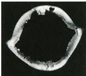
FIGURE 10. CT slice of Bronze Age Iranian portrait head, revealing bands of differing densities.
