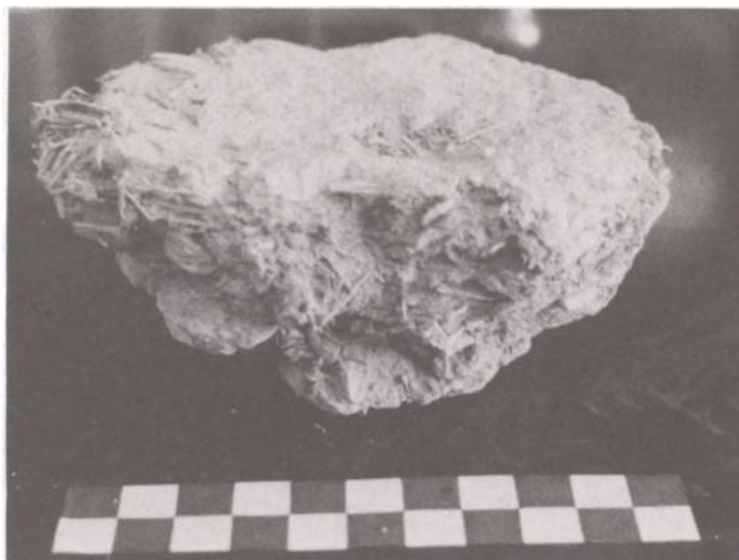
Figure 2: SC1A1 Partial Brick Exposing Straw Binder
