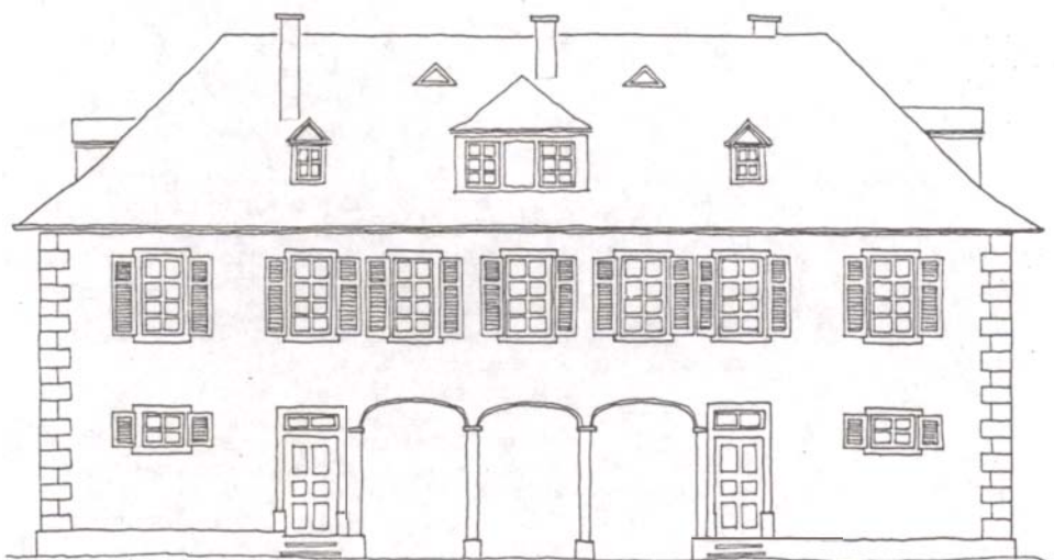
Fig. 10 Princely hotel built of rammed earth 1811 in Fürstenlager near Auerbach-Bensheim. [3]
