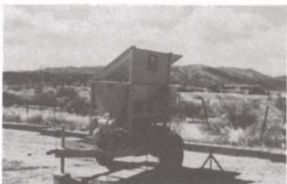
Figure 3. Earth Press III pressed-earth-block machine manufactured near Grants, New Mexico, and set up near a wall under construction in Velarde, New Mexico.
