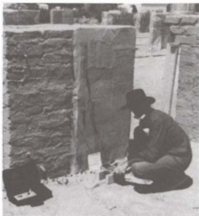
Figure 13. Photograph of control wall (#40) with thermocouples hooked up to data logger for exterior surface and internal temperature monitoring.
