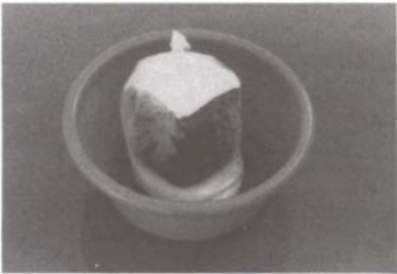
Figure 6. Consolidation test using 4% WS-24 on mud brick.
