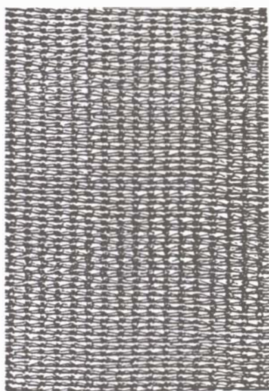
Figure 14. Structure of aerotextile material with 70% shade density.
