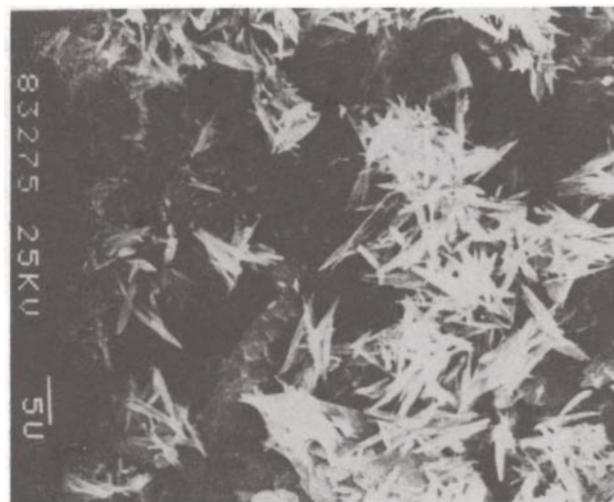
Fig 9 SEM photograph of PS-C, 9000 x.
