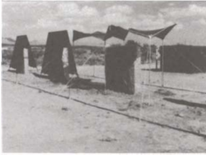
Figure 16. Photograph showing adobe test walls (#38, 39) protected by A-frame, aerotextile-covered shelters, and (#37) by hexagonal shaped 'puckered' shelter with aerotextile roof.
