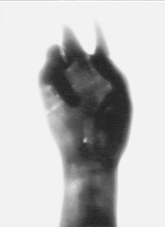
15. The Getty Bronze , x-ray of hand showing that it is solid cast.
