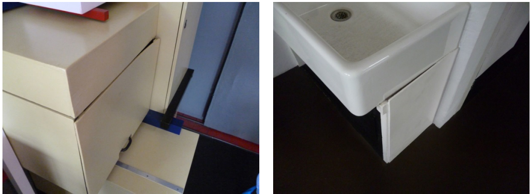
Figure 5: Deformation of thin timber elements of furniture
