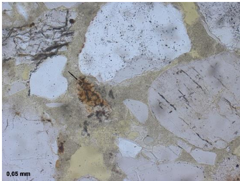
Fig. 17. Microphotograph showing one of the scarce, iron-bearing, belites (indicated by a small arrow) in the binder matrix of the inner mortar in sample RSH 18/3 (TNO 01865, plane polarized light).
