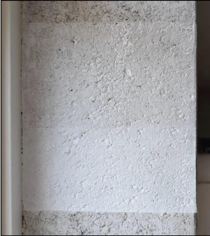
Figure 41. Brushed-on Type S limewash test patch with one (above) and two (below) coats.
