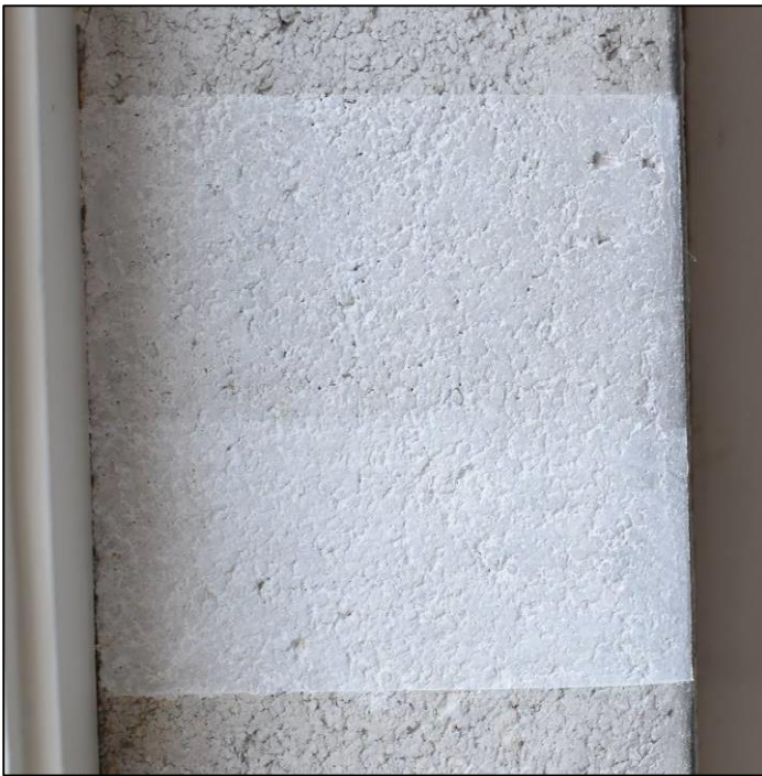
Figure 42. Brushed-on Acrylic-modified Type S limewash test patch with one (above) and two (below) coats.
