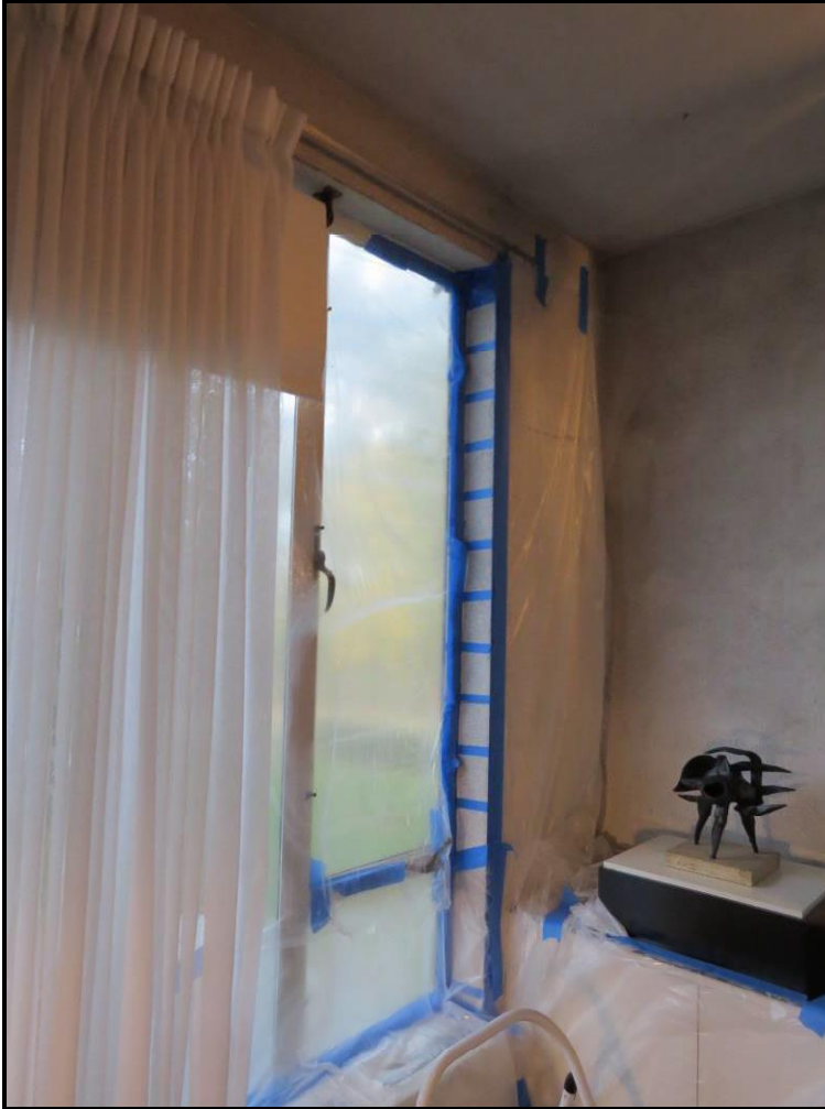
Figure 23. Location of cleaning test patches (marked in blue tape) on window return in living room.
