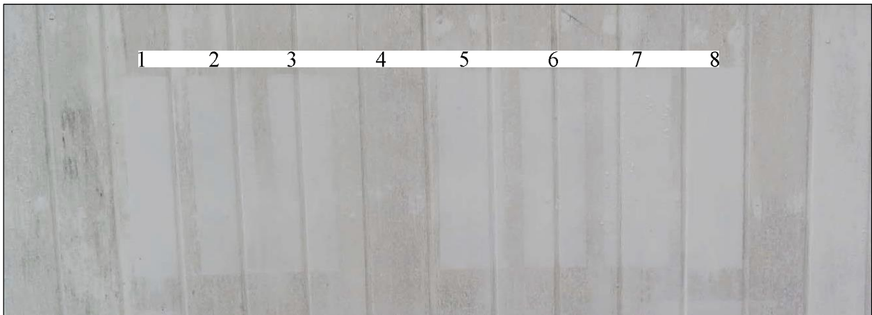
Figure 18. Cleaning test area on west elevation of roof deck after application. Products: (1) 1.25% Sodium Hypochlorite, (2) Water, (3) Wet & Forget, (4) [untreated], (5) Vulpex, (6) Orvus, (7) D/2, (8) 5% Sodium Hypochlorite.
