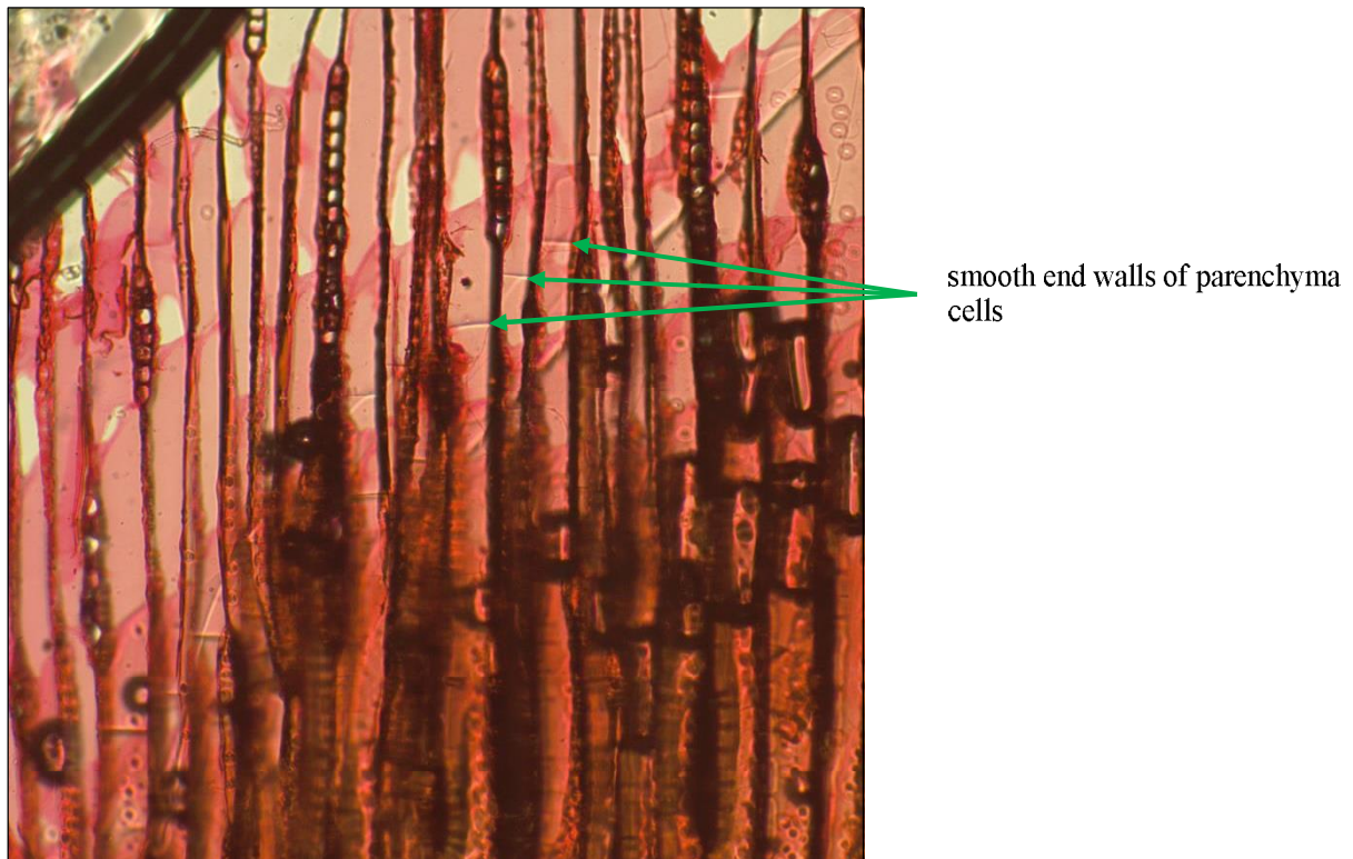
Figure 6. Stained and mounted tangential section of wood sample GH-W-04. (100X)
