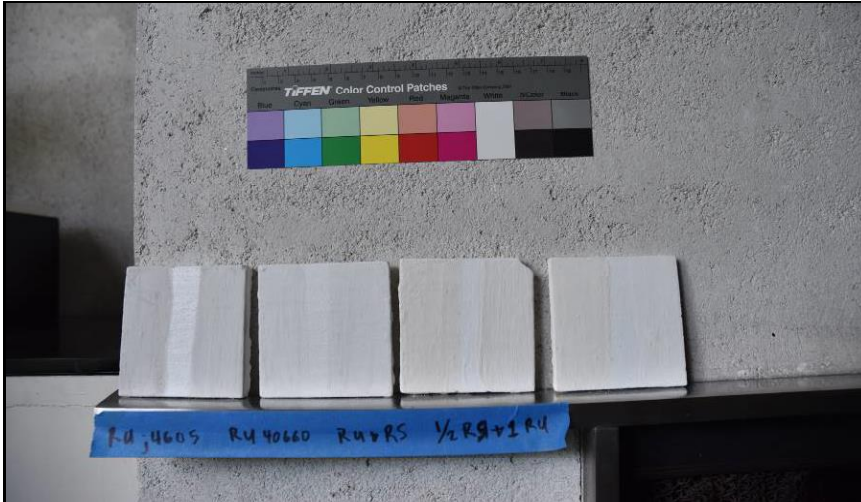
Figure 46. Tinted limewash samples (prepared off-site) compared to plaster above living room fireplace mantle (sample at far left selected for test).
