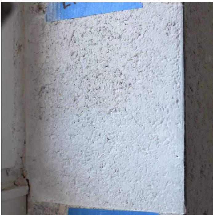
Figure 40. Brushed-on acrylic-modified lime putty limewash test patch with one (above) and two (below) coats.
