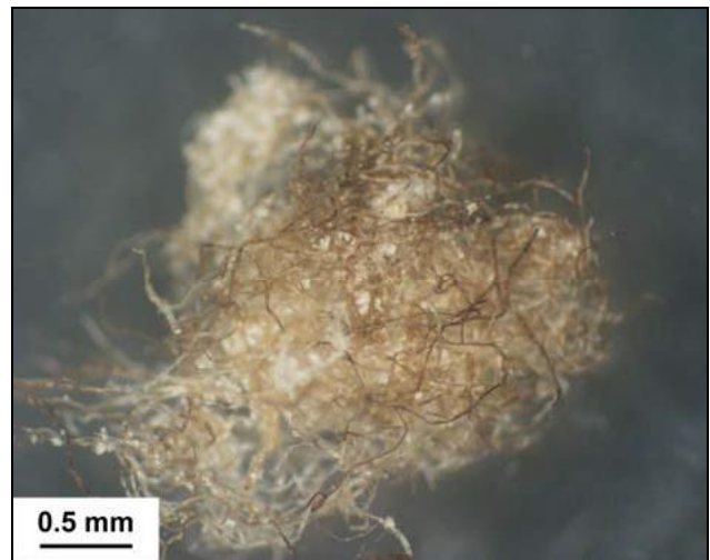
Figure 5: (Upper XPL image) The binder (B) is homogeneous with a low birefringence and appears to consist solely of hydrated lime. Undispersed lime grains (L) are relatively common. The arrows indicate fine fibers that are embedded in the binder. (Lower left reflected light image) The fibers were extracted from the binder through acid digestion. A tangled mat is shown on a filter paper in the same manner it existed within the plaster. Note that most of the fibers are white and difficult to distinguish against the similarly light background. A few red and blue fibers are also detected. (Lower right reflected light image) The fibers were fired at relatively low temperature. Note the charring that indicates the fibers are not mineral based.
