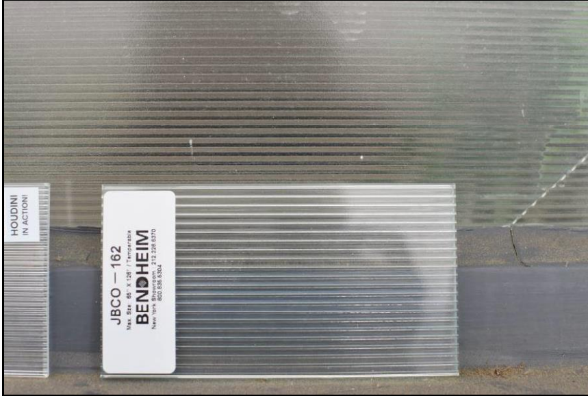
Figure 16. Sample of Bendheim's JBCO-162, "ribbed" glass compared to original glass in Window 102 (south elevation).
