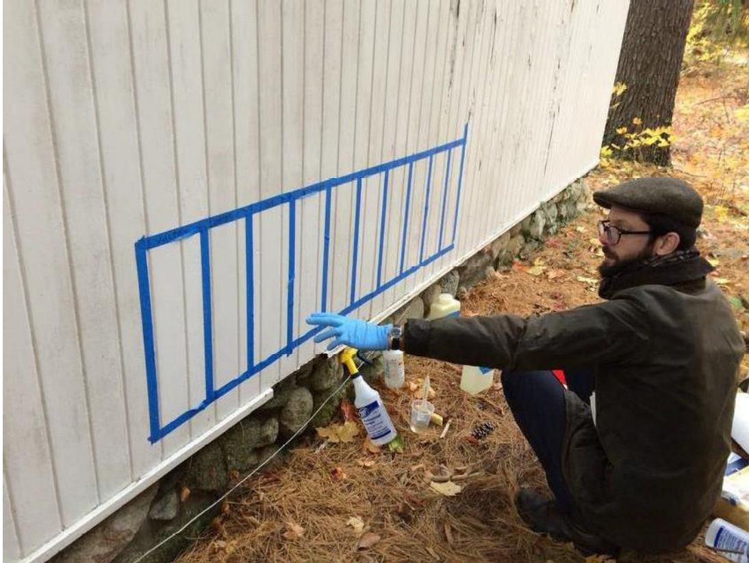
Figure 7: Ed Fitzgerald of JBC tests cleaning solutions for the siding, 2015 RS ID #265422
