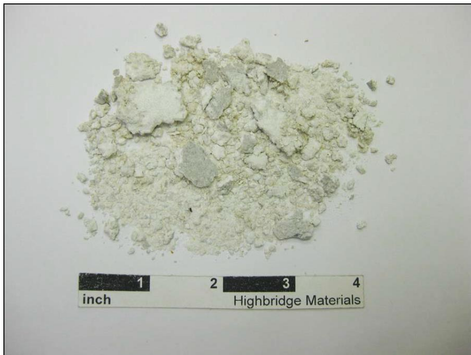
Figure 1: Photograph of the sample provided to Highbridge for examination. The acoustical plaster is nearly white except where soiled to a light gray color.
