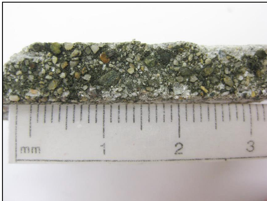
Figure 1: Photographs of the mortar sample provided to Highbridge for examination. The mortar is uniform in appearance with a gray color. The cured product is hard, nonfriable, and not noticeably water absorptive. The lower image shows a closer view of the tooled surface. The exposed aggregate contributes some color and textural variegation to the weathered joint face. However, the overall color is much darker than the fresh paste due to soiling at the surface.
