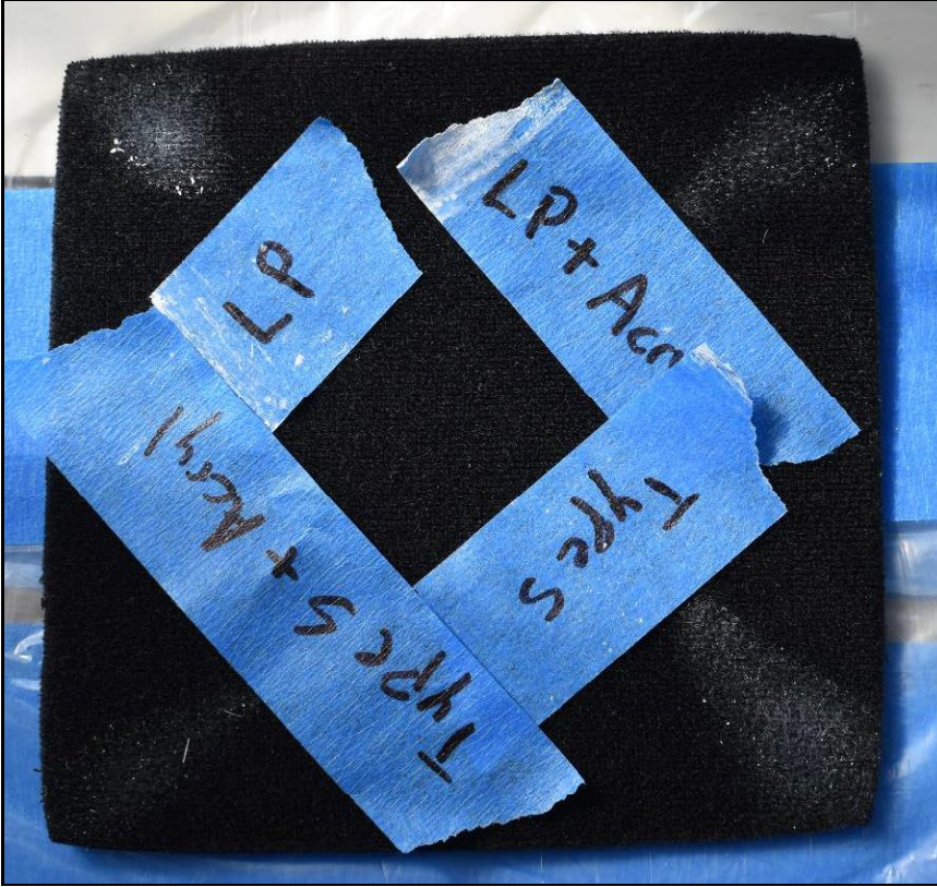
Figure 45. Chalking test cloth with residue from brush applications of (clockwise from top left corner) lime putty, acrylic-modified lime putty, Type S, and acrylic-modified Type S limewash variations.
