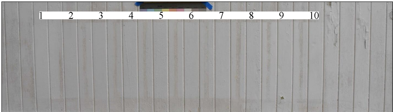
Figure 15. Cleaning test area on east elevation of garage after application. Products: (1) Vulpex, (2) Water, (3) D/2, (4) Wet & Forget, (5) TSP, (6) 3% Hydrogen Peroxide, (7) 30% Hydrogen Peroxide, (8) 1.25% Sodium Hypochlorite, (9) 5% Sodium Hypochlorite, (10) Orvus.
