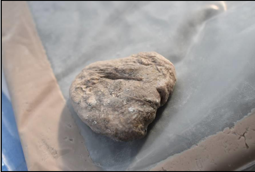
Figure 37. Groom/Stick after use. Note darker color of used product (center) compared to unused product in packaging (left). Also note white plaster fragments embedded in used product.
