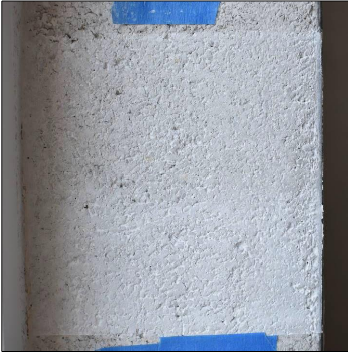
Figure 39. Brushed-on lime putty limewash test patch with one (above) and two (below) coats.
