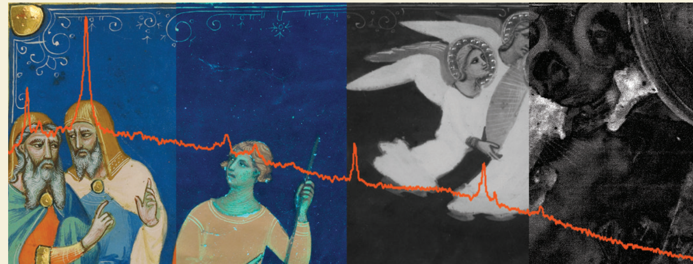
Composite visualization of four images (visible, UV, infrared, and x-ray images) and spectroscopic data from adjacent areas of a single fourteenth-century manuscript leaf (JPGM collection, Ms. 80b, verso)
