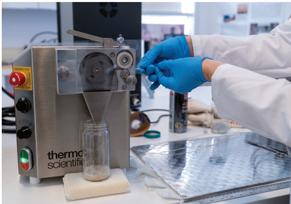
Right: A strand of cellulose acetate plastic is fed into the pelletizer, which chops it into identical pieces. Photo: Andrzej Liguz
