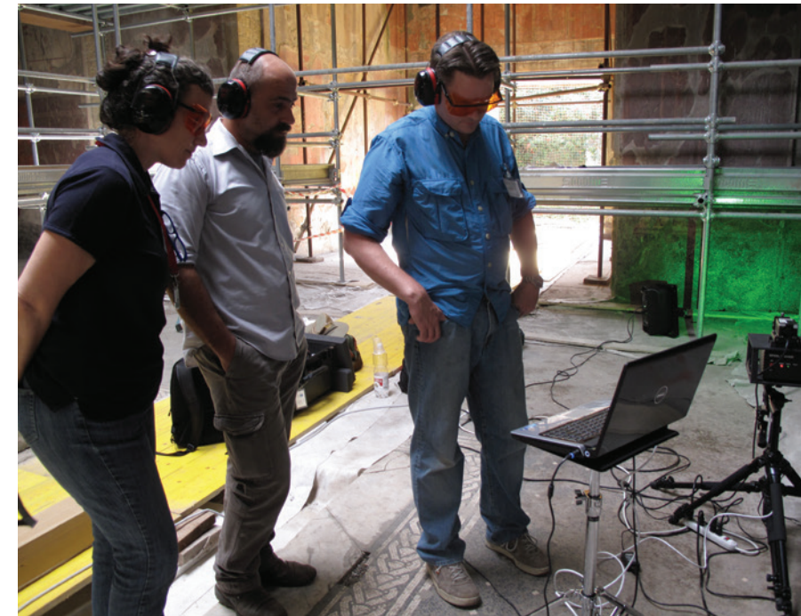
GCI scientists and an HCP specialist use laser speckle interferometry in the House of the Bicentenary to assess specific conditions of the wall paintings and plasters.
