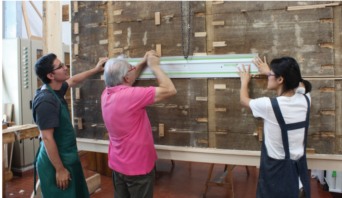
Conservators setting up the router guide tracks in order to re-join the panels. Photo: Britta New, National Gallery, London
