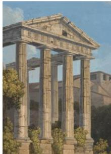
**Column:** an upright post, usually square, round, or rectangular (an example can be seen on the left). It can be used as a support or attached to a wall for decoration. In classical architecture, columns are composed of a **capital**, shaft, and a base (except in the Doric order).
