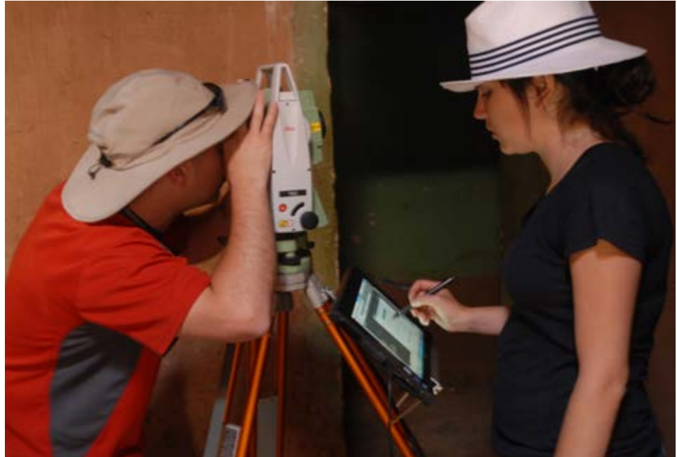
FIGURES 2.23 AND 2.24 CIMS team members recording points using the total station. Photos: Claudia Cancino, 2012.
