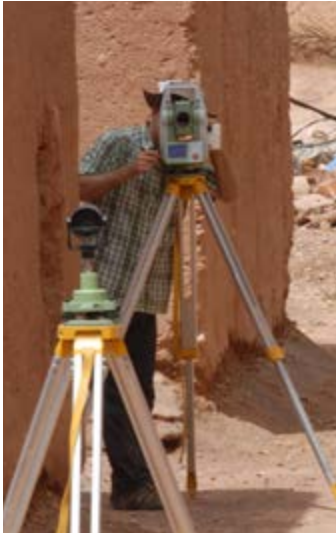
FIGURES 2.23 AND 2.24 CIMS team members recording points using the total station. Photos: Claudia Cancino, 2012.
