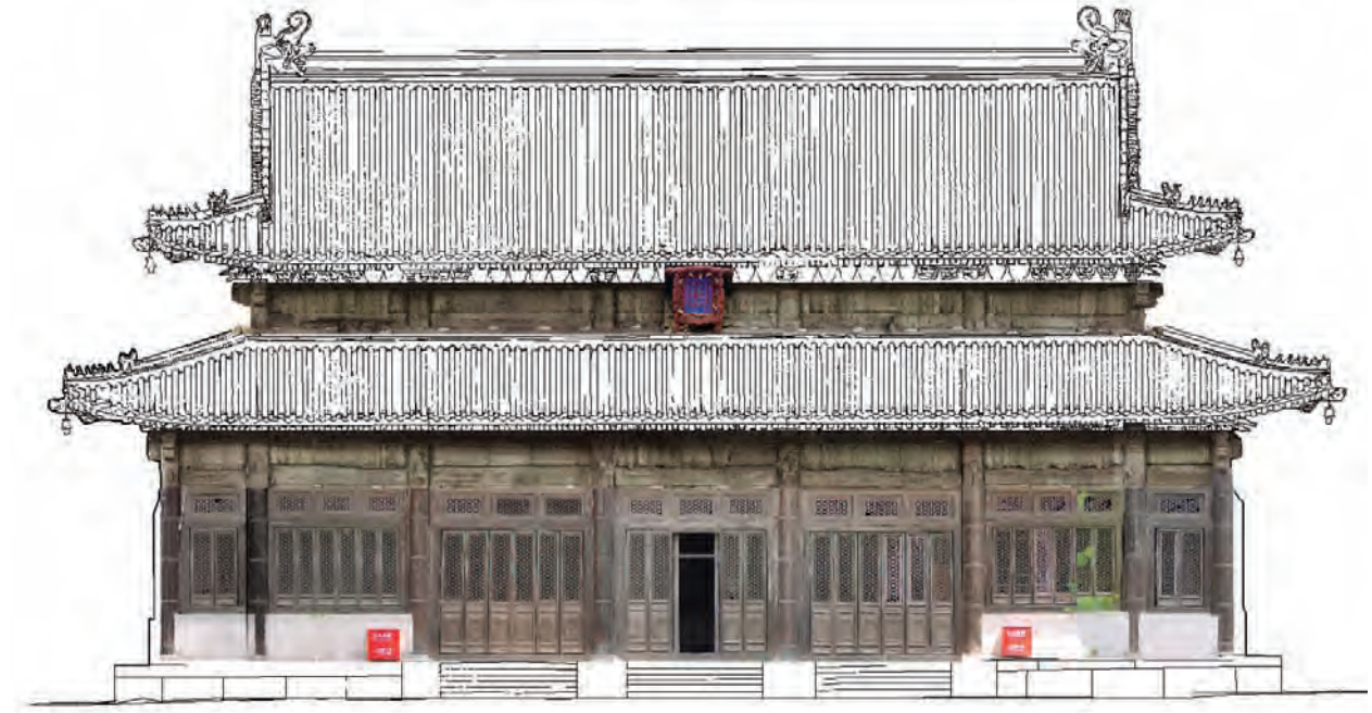
58. 与照片重叠的会乘殿正立面图（南立面） Elevation of Huicheng Hall with partial photographic overlay, South facade
