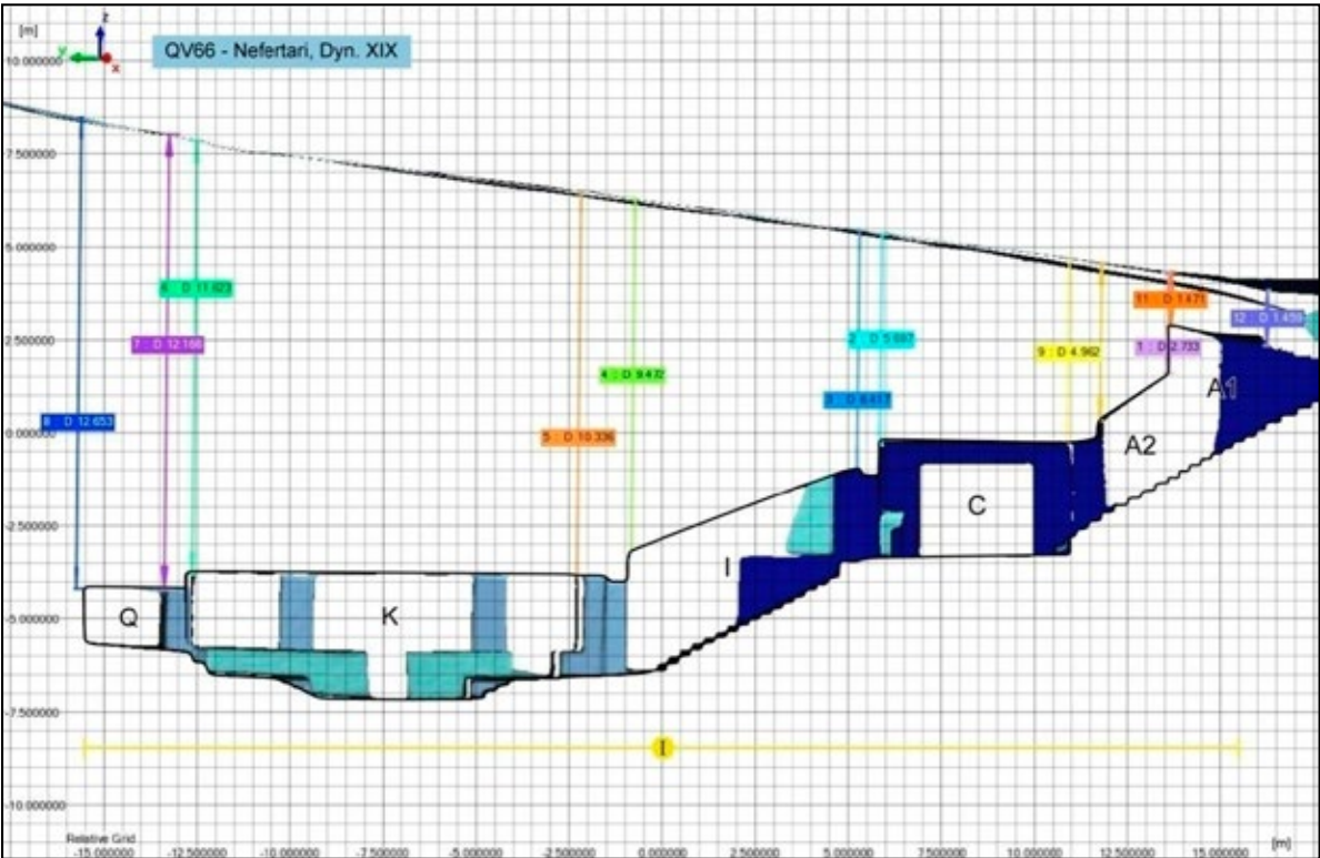
Overburden analysis shows the thickness ranges from 4.96m above chamber (C) to 11.6 meter above burial chamber (K)
