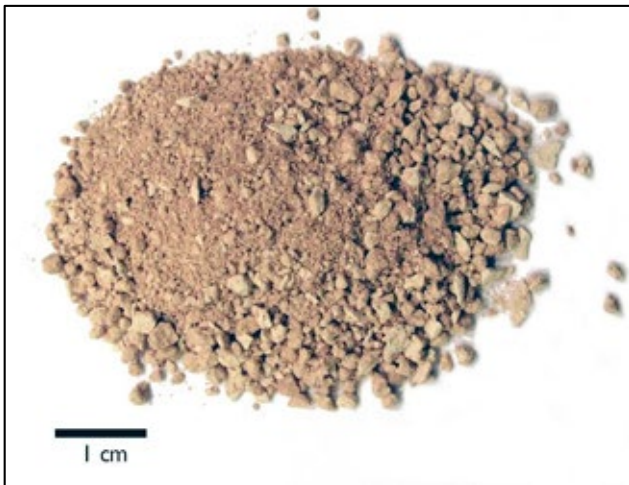
Sample of hiba , a clay-containing calcitic soil, from a deposit in Queens Valley. Many of the tomb plasters were found to be primarily hiba -containing.
