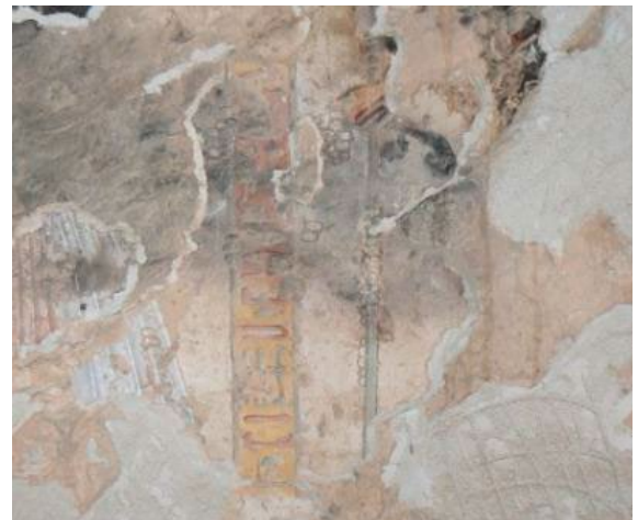
Heat alteration of pigments from yellow to red is also visible.
