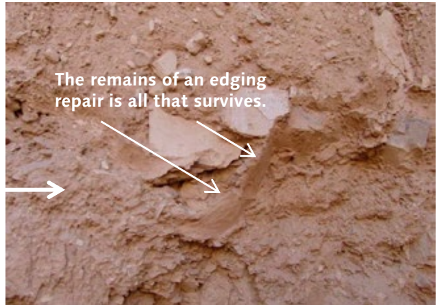
Traces of an edging repair still survive though the painting it once supported has now been lost.
