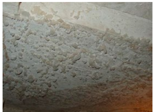
Fibrous salt crystal growth on rock.
