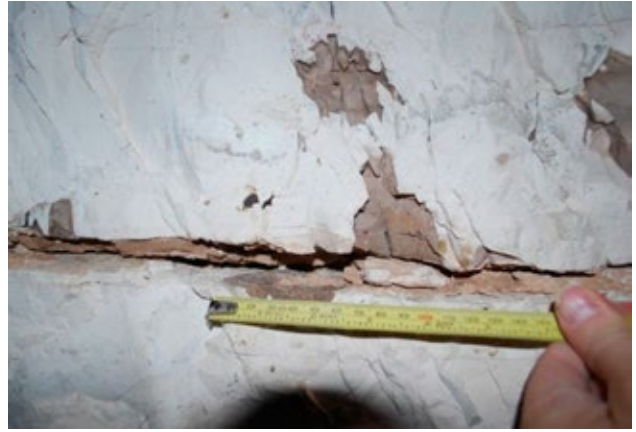
Lateral displacement of chert nodule divided by fissure indicates movement along the fault plane mentioned above.
