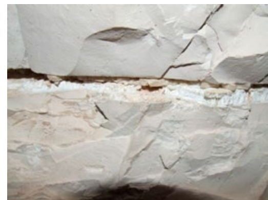
Detail of salt infill in fracture. Analysis identified the upper, darker layer as calcite and the lower, white material as anhydrite.
