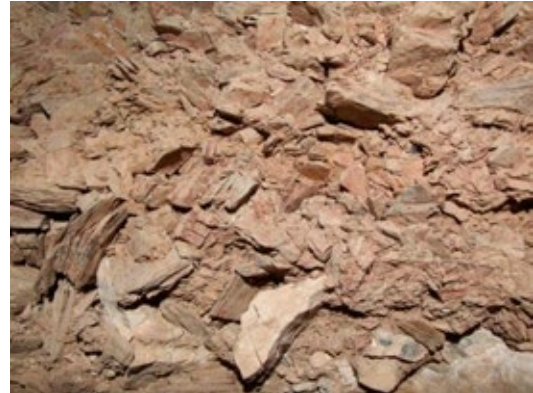
Detail of cemented breccia.
