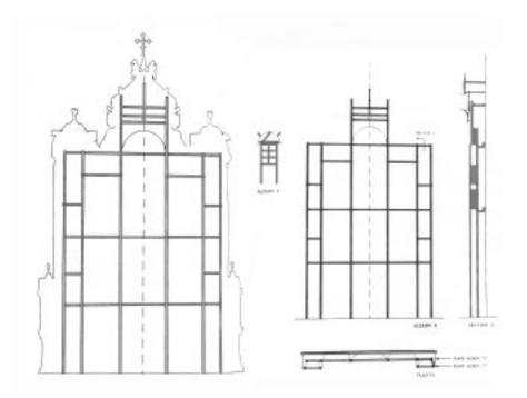
Supporting structure and anchoring system of the altarpiece.
