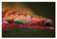
Chemical staining test with Fascina acid and analysis of cross-section stratigraphy (24-98/A-4) revealed the presence of proteins in the preparation layer (above).
