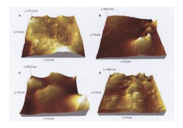
**FIGURE 5** AFM images (3  $\mu$ m × 3  $\mu$ m ) of before-immersion film surfaces: (A) Naphthol Red, (B) Bone Black, (C) Ultramarine Blue, (D) Rhoplex AC-234 film. (Rhoplex AC-234 films were softer, and it was more difficult to obtain good AFM images.)
