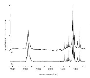
**FIGURE 8** Comparison of FTIR spectra from (A) water extract residue from the surface of the naturally aged sample, (B) reference sample of Triton X-405. The absorbance axis has been offset to assist in comparison.
