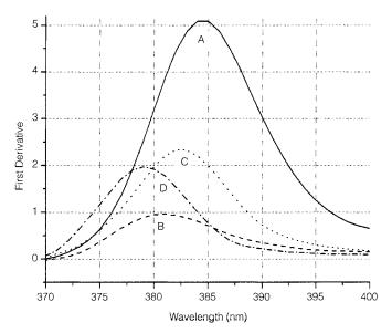
**FIGURE 3** First derivative of the reference white mock paintings' reflectance spectra in the 330–420 nm range: (A) lead white (solid line), (B) zinc oxide (dashed line), (C) lithopone (dotted line), (D) anatase (dash-dot line), (E) rutile (dash-dot-dot line).
