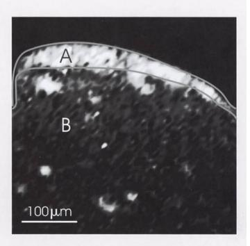
**FIGURE 2** Transmission FTIR image (2940–2850 cm<sup>-1</sup>) of a thin section of the affected paint showing (A) a layer of oil-derived oxidation products on top of (B) the paint layer. Areas of white correspond to high levels of absorbance.
