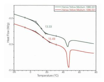
**FIGURE 3** Glass transition temperatures, as measured by modulated differential scanning calorimetry, for Golden Hansa Yellow Medium. Upper curve represents a paint made in 1986; lower curve represents a paint made in 1996.
