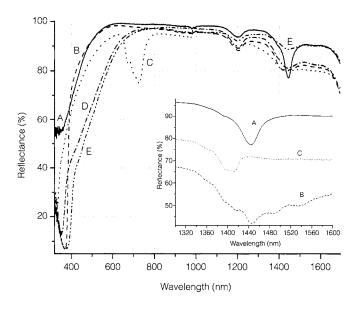
PIGURE 2 Reflectance spectra of the reference white mock paintings in the 320–1700 nm range: (A) lead white (solid line), (B) zinc white (dashed line), (C) lithopone (dotted line), (D) anatase (dash-dot line), (E) rutile (dash-dot-dot line).
