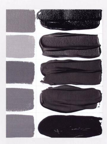
FIGURE 2 Black paints (from top to bottom): Golden Fluid, Guardi, Kreul Solo Goya Acrylic Pastos, Kreul Solo Goya Acrylic Fluid, and Kruel Solo Goya Triton (cracks), with addition of white impasto.
