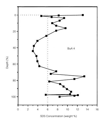
FIGURE 5 Concentration profiles of sodium dodecyl sulfate (SDS) surfactant molecules (an anionic surfactant) in an acrylic film (butyl acrylate/acrylic acid [96:4) copolymer) determined by confocal Raman microspectrometry. Average surfactant concentration was 6% by weight; air at 0% depth; substrate (polyethylene) at 100%. (Belaroui et al. 2003, reprinted with permission.)
