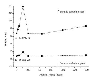
**FIGURE 6** Ratios of the band areas for the acrylic ester peak at 1731 cm $^{-1}$  and two surfactant ether peaks at (A) 1343 cm $^{-1}$  and (B) 1109 cm $^{-1}$  from  $\mu$ ATR-FTIR measurements of the surfaces of artificially aged films of Rhoplex AC-2235. Dashed lines indicate trends suggested by the data. Increasing ratio indicates reduced surface surfactant, whereas a lower ratio signifies increasing concentration of surfactant on the surface.
