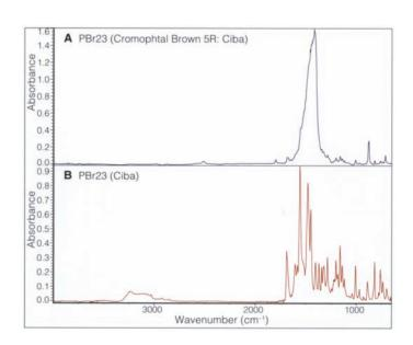
**FIGURE 3** Infrared spectrum of PBr23: (A) sample with CaCO<sub>3</sub> filler, (B) sample of pure pigment.
