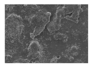
**FIGURE 4** SEM image (1500× magnification) of a sample of blue paint from Jasper Johns's *Untitled* triptych showing crystal-like structures on the surface.
