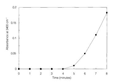
**FIGURE 3** Absorbance at 3400 cm<sup>-1</sup> versus time after water introduction into the cell (values taken from spectra of figure 2).
