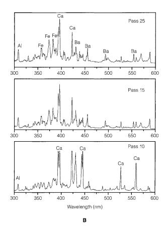
**FIGURE 4** LIBS analysis during cleaning of the AXA Reinhardt painting: (A) Square 8, laser pass 4: presence of Co, Cu, and Al. Square 8, laser pass 8: presence of Fe indicates breakthrough into an iron-rich layer. (B) Square 2: increase in Fe as the laser penetrated the first iron-rich layer. Illustration: Kristalia Melessanaki, IESL FORTH.
