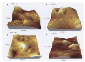
**FIGURE 6** AFM images (3  $\mu m \times 3~\mu m$ ) of after-immersion film surfaces: (A) Naphthol Red, (B) Bone Black, (C) Ultramarine Blue, (D) Rhoplex AC-234 film. (Rhoplex AC-234 films were softer, and it was more difficult to obtain good AFM images.)
