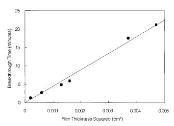
**FIGURE 5** Water breakthrough times for Liquitex acrylic gesso films (data from fig. 4) plotted against the square of the film thickness. The slope of the fitted line is related to the diffusion coefficient by the equation slope  $= 1 / (6 \times \text{diffusion coefficient})$ . The R<sup>2</sup> value for the least-squares fit is 0.99.
