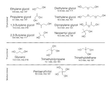
**FIGURE 3** Structures and relevant chromatographic information for polyols commonly formulated into alkyd resins. Listed below the molecular structures are the retention time of the trimethylsilyl ether derivative and the ion used for GC/MS quantification.
