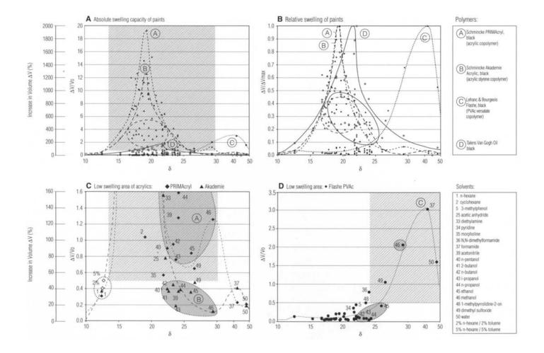
FIGURE 2 (A) The absolute swelling values of latex paint films on immersion in solvents spread along the polarity scale.
