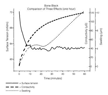
**FIGURE 1** Rate of leaching and swelling for Bone Black paint films. Surface tension, conductivity, and swelling rates are compared.
