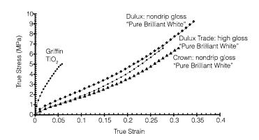
FIGURE 6 Stress-strain curves for white alkyd paints.
