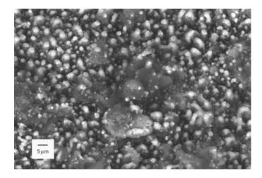
**FIGURE 5** SEM image of cone structure on surface after laser cleaning of the overpainted areas.
