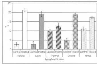
**FIGURE 3** DSC analysis—the effect of aging, modification, and 1-hour water immersions (treated) on  $T_{\rm g}$  (Liquitex Titanium White free films).
