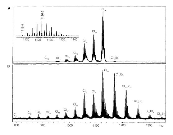
FIGURE 1 LDI-MS spectra of phthalocyanine green PG7 from
