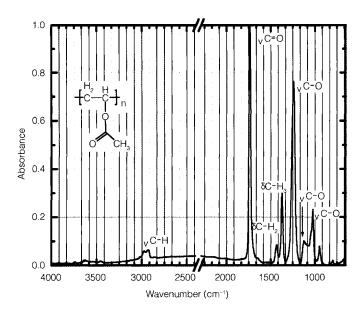
**FIGURE 6** FTIR spectra of polyvinyl acetate homopolymer from Sigma Aldrich (MW 83000), obtained with a diamond compression cell, in a Continuµm-Nexus from Nicolet microFTIR.
