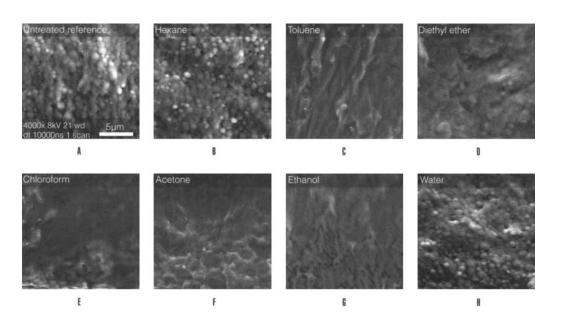
electron mode) of freeze-fractured surfaces showing the inner microstructure of an acrylic latex film. The influence of seven solvents spread across the polarity scale is visualized, showing varying degrees of destruction of the morphological structure.
