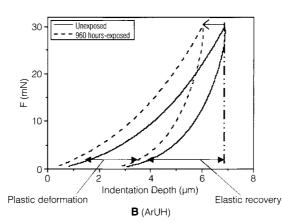
of acrylic-urethane paint films. Change in the loading-unloading curves for the effect of accelerated UV aging: (A) aliphatic urethane, no light stabilizers; (B) aromatic urethane, light stabilizers added. (Adapted from Lee and Kim 2006, with permission.)
