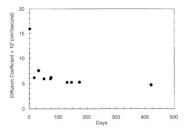
**FIGURE 6** Water diffusion coefficients for films of Liquitex acrylic gesso ( $610-685 \mu m$  thickness) measured at various times after film preparation.
