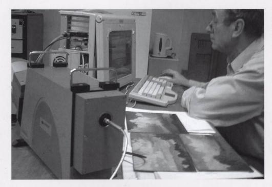
FIGURE 1 Using the LIBS Mechelle spectrometer with iStar DV434 camera to make in situ measurements on paintings.
