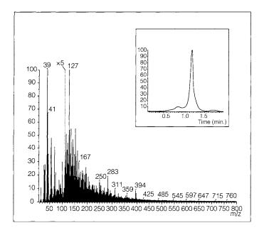
FIGURE 8 DTMS of Golden acrylic paint containing PY3.
