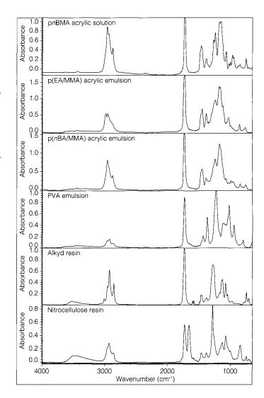
**FIGURE 9** FTIR spectra of unpigmented films of acrylic solution, acrylic emulsion, PVA, alkyd, and NC resins.
