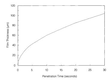
**FIGURE 7** Calculated water penetration time for an artists' acrylic coating film having a diffusion coefficient of  $5 \times 10^{-7}$  cm<sup>2</sup>/second.
