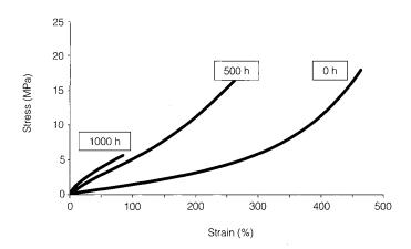
**FIGURE 1** Effects of accelerated light aging (xenon lamp,  $\lambda > 295$  nm) on the stress-strain curves of a Primal (Rohm and Haas) ethyl acrylate—methyl methacrylate copolymer latex acrylic film.
