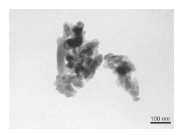
**FIGURE 3** Transmission electron microscope image of some particles of green halogenated copper phthalocyanine pigment, PG7. Note that the primary particles are smaller than the wavelength of visible light.
