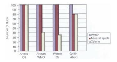
**FIGURE 3** Resistance to water/solvents: double-rub testing of samples painted on glass after curing for two months. Tests stopped at 100 rubs.
