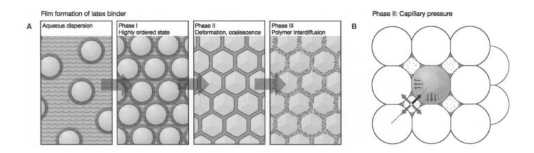
figure 1 (A) In a simplified model, the drying and film formation process can be described by three distinct stages.
