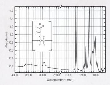
**FIGURE 2** FTIR spectrum of the binding medium from a sample of Sarmento's *Just a Skin Affair*, showing the characteristic absorption bands of polyvinyl acetate.
