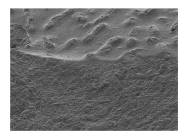
**FIGURE 6** SEM image (1200× magnification) of a sheared sample of cadmium zinc yellow paint from Jasper Johns's *Untitled*, showing a skin of medium on the surface.
