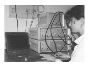
FIGURE 1 Apparatus used for noninvasive, in situ measurements. From top to bottom: xenon light source module, UV-Vis-NIR spectroanalyzer with a tungsten-halogen lamp module, NIR spectroanalyzer module.
