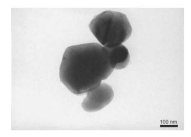
**FIGURE 2** Transmission electron microscope image showing particles of a general-purpose type of titanium dioxide pigment. Less-dense surface treatment layers of silica and hydrated alumina can be seen around the darker core of titanium dioxide.
