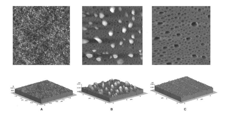
**FIGURE 7** AFM images of an experimental methyl methacrylatebutyl acrylate copolymer film, formulated with 4.6% (by weight) sodium dodecyl sulfate surfactant;  $T_g$  of copolymer = 10° C: (A) dry film, (B) after thermal treatment, 2 hours at 120° C, (C) after thermal treatment and rinsed in water for 5 minutes.
