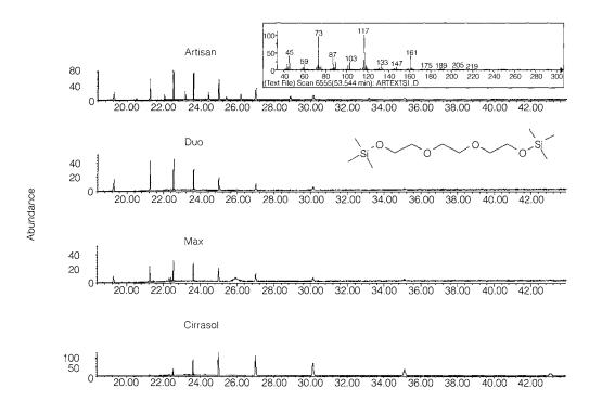
matograms of m/z 161 for three water-mixable oil media and Cirrasol (a POE-based additive). Inset shows the mass spectrum and molecular structure for one of the POE additive peaks.
