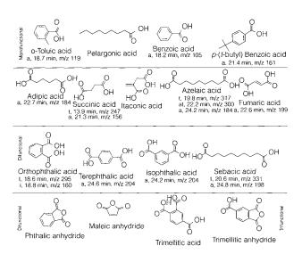
**FIGURE 2** Structures and relevant chromatographic information for polybasic acids commonly formulated into alkyd resins. Listed below the molecular structures are the types of derivative formed (t = trimethylsilyl ester, a = amide, i = imide), retention time, and the ion used for GC/MS quantification. Acids with no data listed cannot be detected by the modified ASTM GC/MS procedure.
