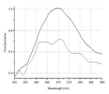
**FIGURE 6** First derivative of the reflectance spectra in the 350–390 nm range of the reference anatase (solid line) and the white spot from the Pitré self-portrait (dashed line).
