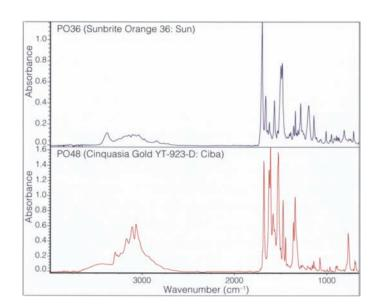
FIGURE 2 Infrared spectra of PO36 and PO48.
