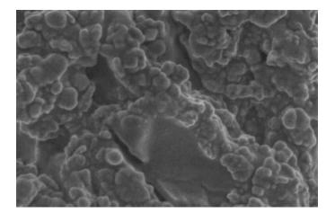
**FIGURE 8** SEM image (70,000× magnification) of aggregated efflorescence on sample of blue paint from Karel Appel's *L'homme*.
