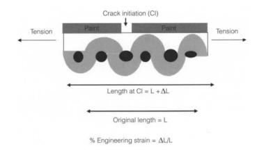
FIGURE 1 Crack initiation.
