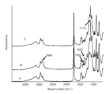
**FIGURE 2** ATR-FTIR spectra of Cryla (Daler Rowney) yellow ochre acrylic color: (A) unaged, (B) naturally aged >5 years, (C) light aged ( $\lambda$  > 400 nm) 32 weeks.
