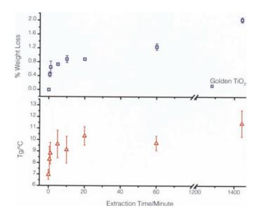
**FIGURE 2** Surfactant extraction: Films of Golden Titanium White were soaked for various periods of time in water. Lower portion shows resulting changes in glass transition temperature  $(T_{\mathfrak{g}})$ . Top portion shows resulting weight loss from the films.
