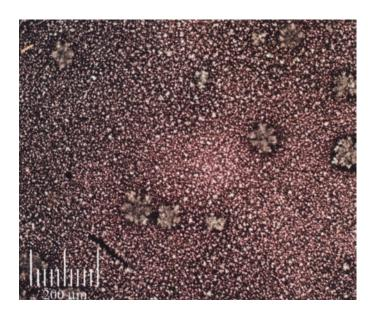
**FIGURE 4** Transmitted polarized light photomicrograph with crossed polarizers of Rhoplex AC-2235 film surface following 1196 hours of artificial aging.
