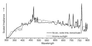
**FIGURE 2** Scaled irradiance spectrum of the Xe arc source filtered by soda-lime and borosilicate glass filters (solid line) compared to unfiltered Arizona sunlight (dashed line). The effect of the window glass filter is seen in the reduced intensity of the arc source below 400 nm.
