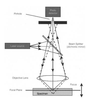
**FIGURE 4** Scheme of confocal Raman microspectroscopy. The broken line indicates the out-of-focus laser light beam, which cannot reach the detector. (Marton et al. 2005; reprinted with permission.)
