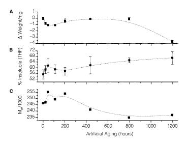
**FIGURE 5** Results for changes in (A) sample weight, (B) percent polymer film insoluble in THF, (C) weight-average molecular weight of the soluble fraction in THF during aging. Dashed lines indicate trends suggested by the data.
