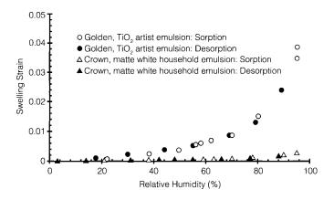
**FIGURE 8** Hygral expansion strains for the Golden and Crown (matte) emulsions versus relative humidity at  $23^{\circ}$  C.
