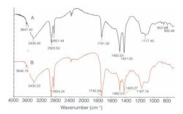
FIGURE 7 FTIR spectra of (A) Jasper Johns's *Untitled* and (B) dried Winsor & Newton Cadmium Yellow Deep paint (ca. 1971). Absorptions at 1740 cm<sup>-1</sup> indicate oil, 1482 and 1421 cm<sup>-1</sup> magnesium carbonate, and 1000–1200 cm<sup>-1</sup> barium sulfate. There was no indication of aluminum stearate or hydroxide.
