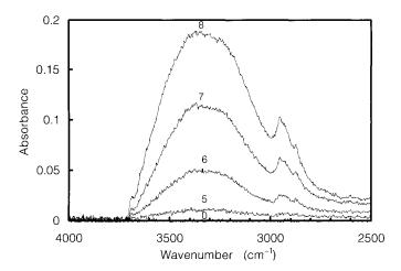
FIGURE 2 Typical infrared spectrum of acrylic coating on ATR crystal, measured at 0, 5, 6, 7, and 8 minutes after water introduction into the cell. Increase in absorbance at 3400 cm<sup>-1</sup> indicates emergence of water through the bottom of the coating film.
