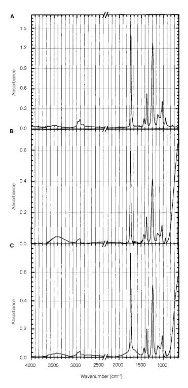
**FIGURE 9** FTIR spectra of Joaquim Rodrigo's white microsamples, obtained with a diamond compression cell for (A) extract of the last white paint left by the artist in his studio; (B) *Port-Ligat—Granada*, 1980; (C) *M.L.*, 1961.
