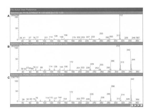
Other organometallic pigments gave good mass spectra as well. In addition to the phthalocyanines described above, PG8, PG10, PY150, and PR257 gave well-defined pyrograms with mass spectra that, in general, did not include a peak for the molecular ion.
