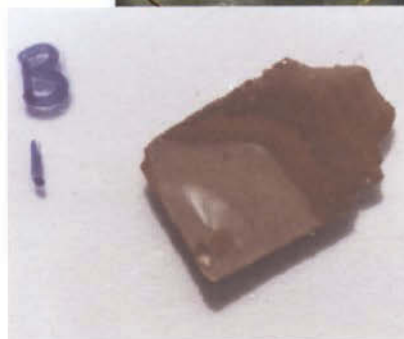
FIGURE 8 a, b Testing plate with coated original tesserae and artificial high-potassium glass (a). Delamination of epoxy coating after eight days of exposure in test chamber (b).
