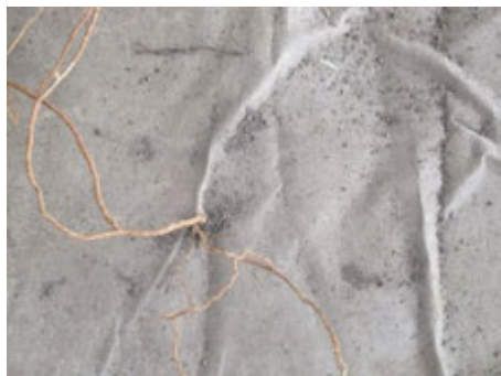
Roots penetrated geotextile in 2 places (left and center); holes may have been created by termites, allowing root access. Small holes created by termites in geotextile (right).
