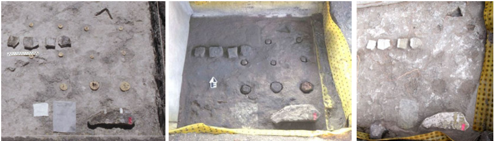
Quadrant 1 as established in 1995 (left), excavated in 1997 (center) and re-excavated in 2011 (right). Weathering and cracking of tuff floor can be seen in the 1995 photo around the geotextile and treated block.
