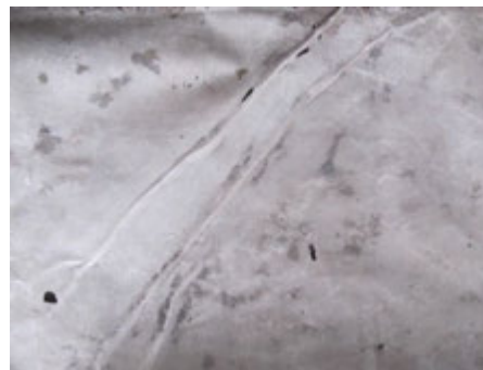
Roots penetrated geotextile in 2 places (left and center); holes may have been created by termites, allowing root access. Small holes created by termites in geotextile (right).
