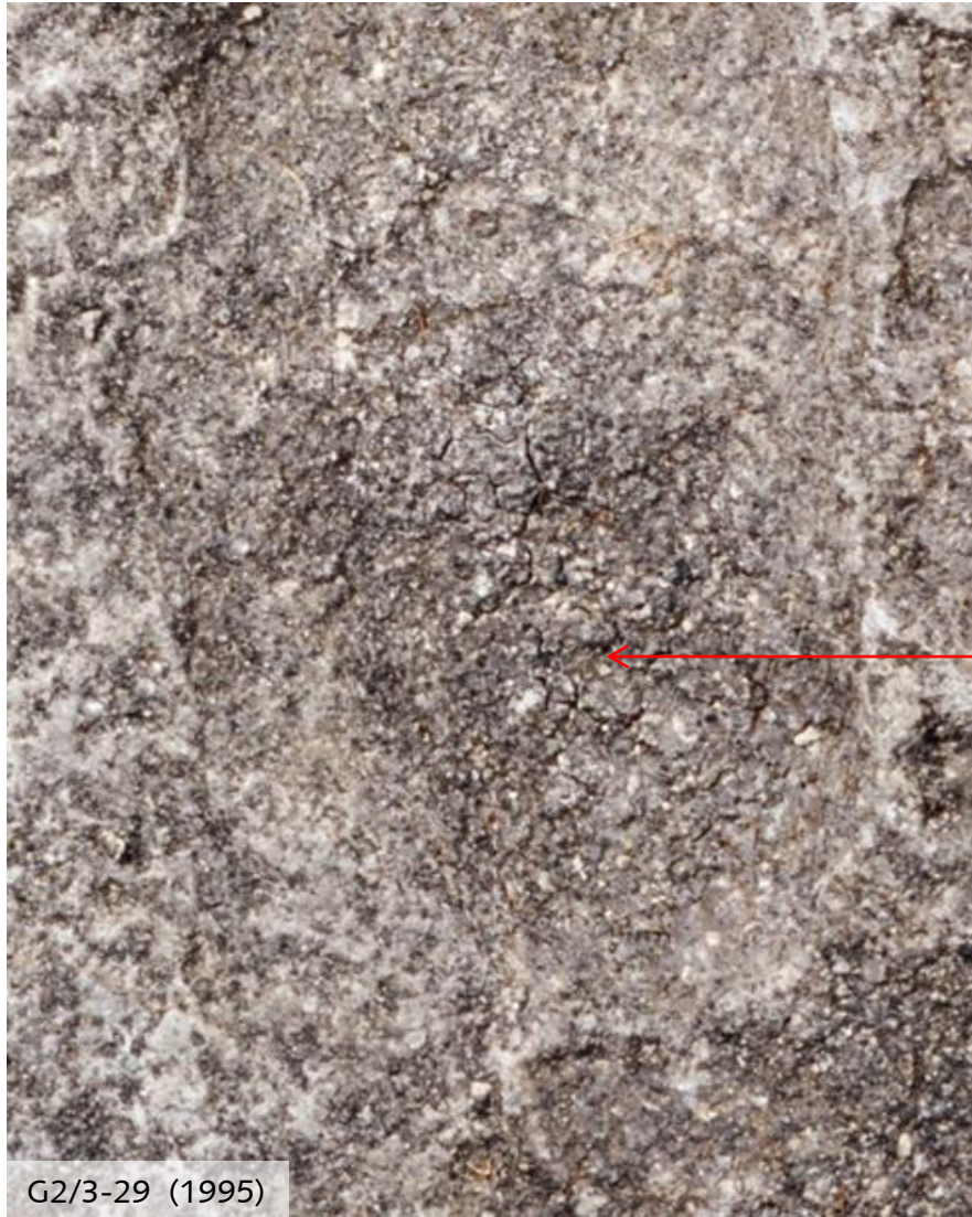
Close-up of heel of G2/3-29 in 1995 and 2011 showing incipient cracking in heel in 1995 slightly enlarged in 2011
