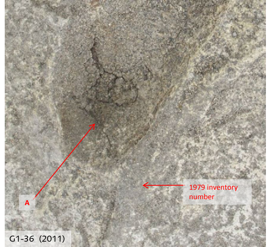
Close-up of the heel of G1-36 in 1995 and 2011. Transverse crack in heel (A) was visible in 1995 and was noted on photos and cast from 1979. Incipient cracking (possibly weathering) in heel recorded in 1995 has increased.
