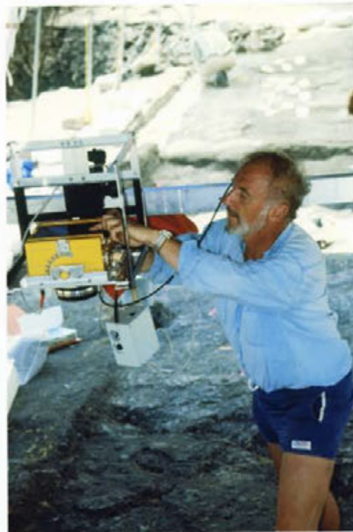
52. UMK camera on crossbar used for photogrammetric recording of the trackway and footprints.
