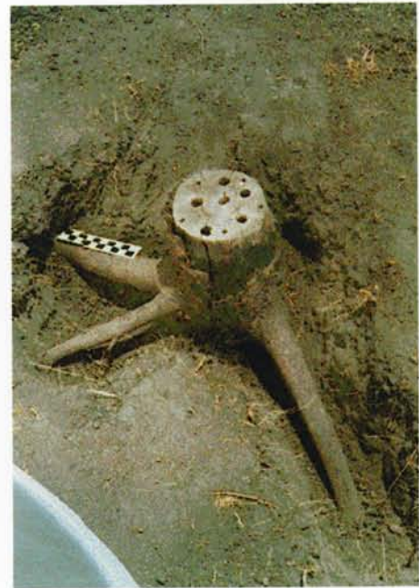
43. Stump tested off-site for efficacy of PCP treatment in preserving wood.
