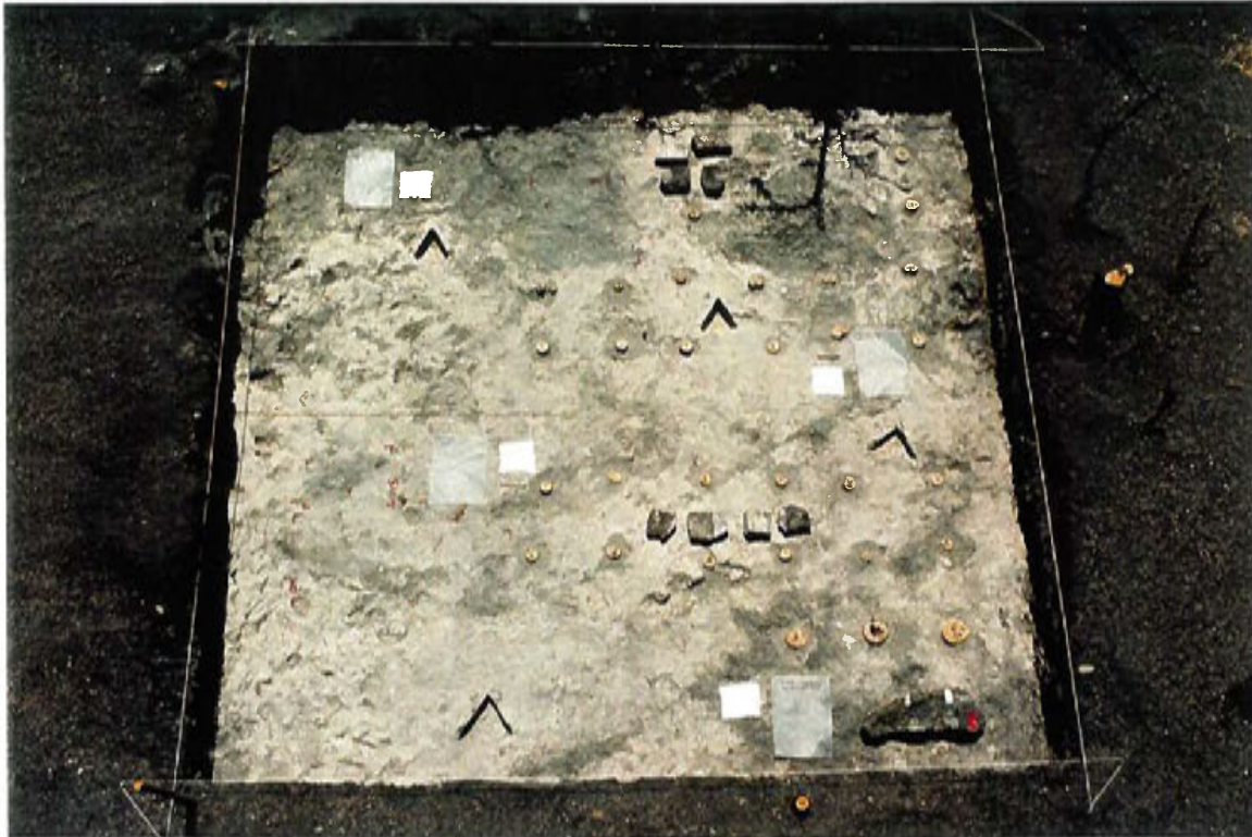
36. Test Site 3. Placement of duplicate test samples in the north (top) and south (bottom) sections of the reburial monitoring trench.
