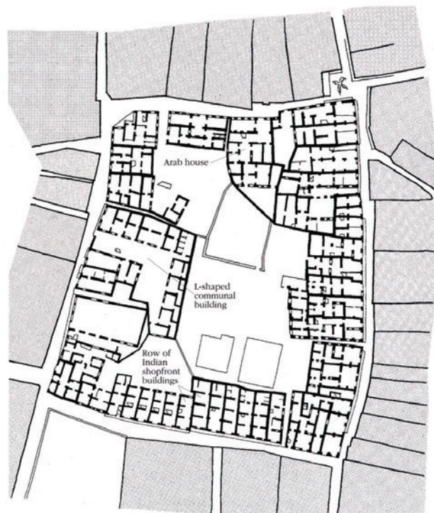
Plan of an urban block in the Kajificheni neighborhood. This typical block contains a mix of building types, including Arab houses, groups of Indian shopfront buildings, and an L-shaped communal tenement structure. Drawings: R. Marks © The Aga Khan Trust for Culture.
