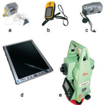
Fig. 53 Tools for heritage recording: (a) measuring tape and plumb line, (b) electronic distance meter, (c) digital camera, (d) Tablet PC, (e) total station. Photos: Rand Eppich.
