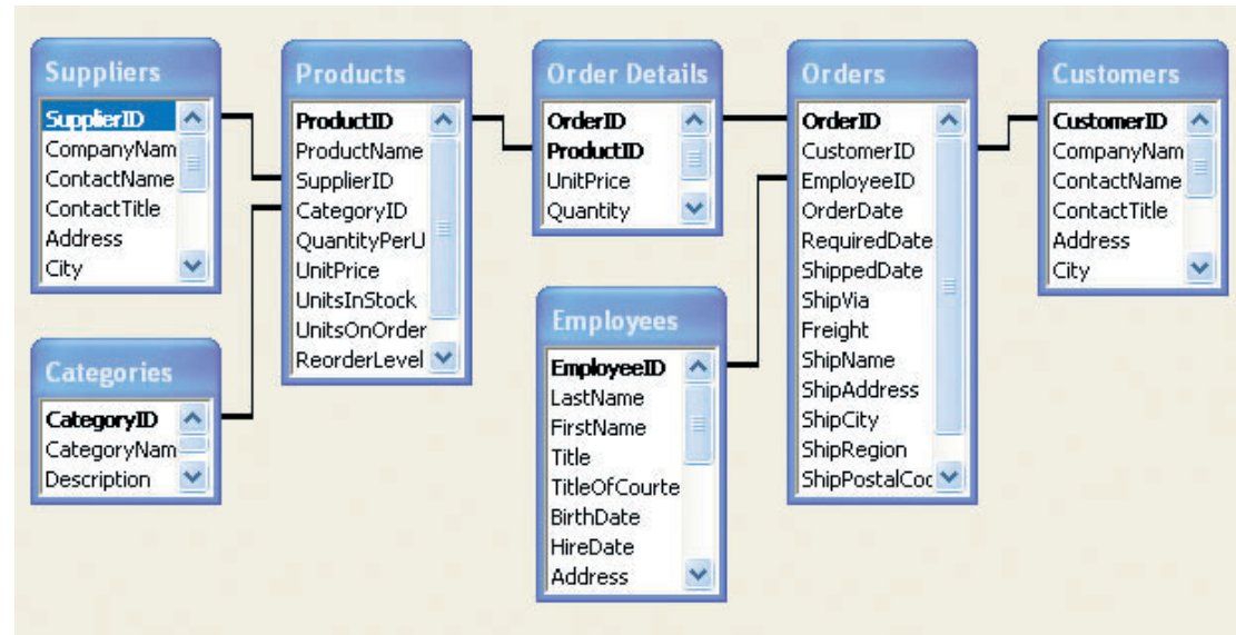
Fig. F.1 Example of a relational database. The relationship between the “Suppliers” and “Products” tables is the SupplierID, a unique number that is identical in both tables. The relationship between the “Products” and “Order Details” tables is the ProductID number.
