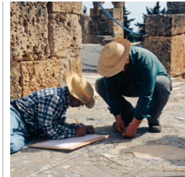
Fig. 44 Technicians conducting a measured site survey at an ancient Roman mosaic site in Tunisia. A survey can be carried out by a team of archaeologists, architects, or technicians using simple recording tools, such as a water level, plumb line, and measuring tape. An advantage of producing measured drawings by hand recording is prolonged direct contact with the object, which allows for thorough analysis. Photo: Bettina Lucherini.
