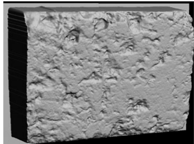
FIGURE 18 Three-dimensional surface model derived from stereophotographs.
