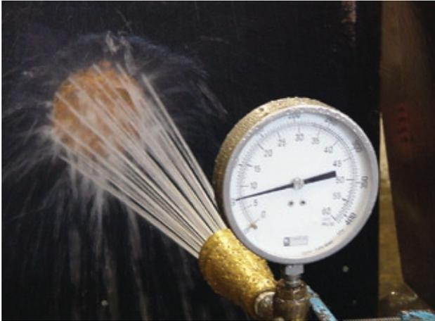
FIGURE 13 Accelerated degradation water spray test.
