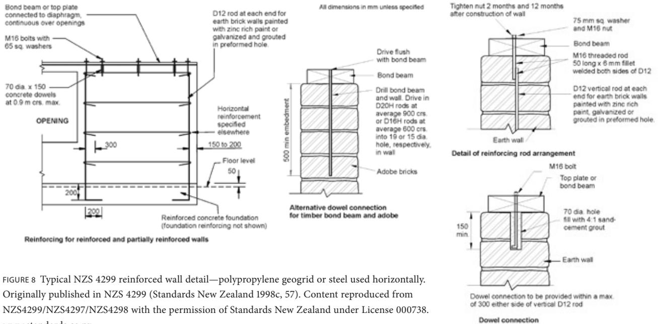
FIGURE 8 Typical NZS 4299 reinforced wall detail—polypropylene geogrid or steel used horizontally. Originally published in NZS 4299 (Standards New Zealand 1998c, 57). Content reproduced from NZS4299/NZS4297/NZS4298 with the permission of Standards New Zealand under License 000738. www.standards.co.nz.
