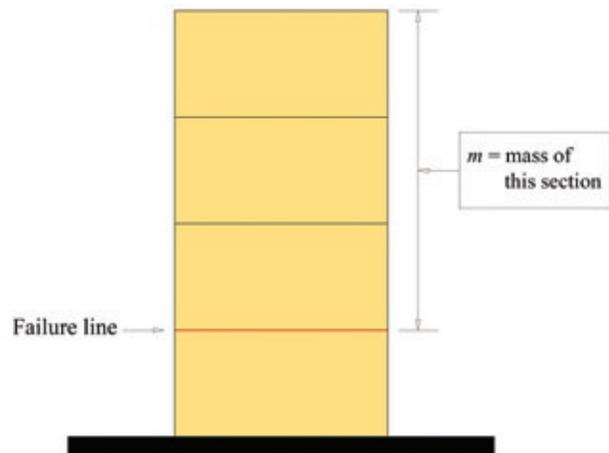
FIGURE 13 Description of mass used for calculating cohesion.
