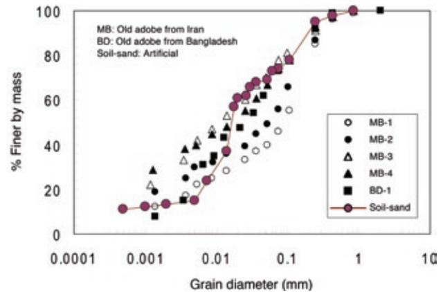
FIGURE 1 Grain size distribution of the soil-sand mixture.
