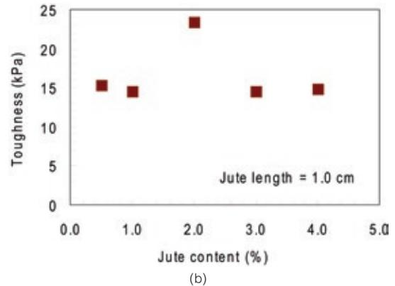
FIGURES 5A AND 5B Typical stress-strain relationships of jute-reinforced adobe (a), and variation of toughness with jute content (b).
