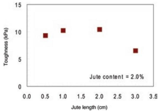
FIGURE 6 Variation of toughness with jute length.
