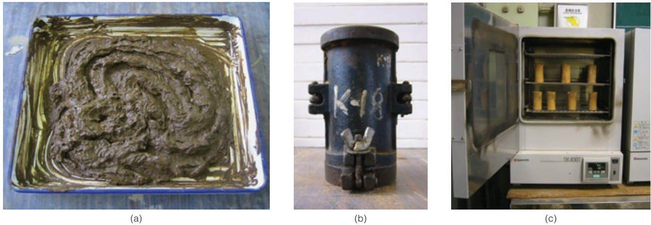
FIGURES 2A-C Preparation of adobe specimens: soil-sand slurry (a); steel mold for specimen preparation (b); and oven used for drying specimens (c).
