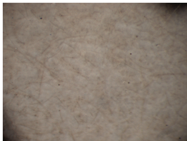
Figure 10b Detail of the Dmin area of the photograph in fig. 6 at 80x magnification, showing fibers in the paper substrate.
