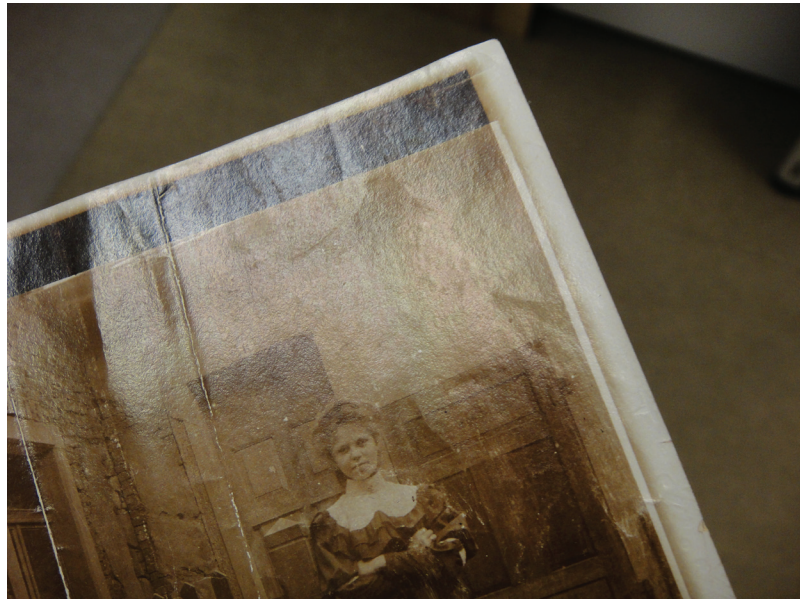
Figure 7 Glossy collodion photograph displaying a typical interference color pattern when held up to a light source.
