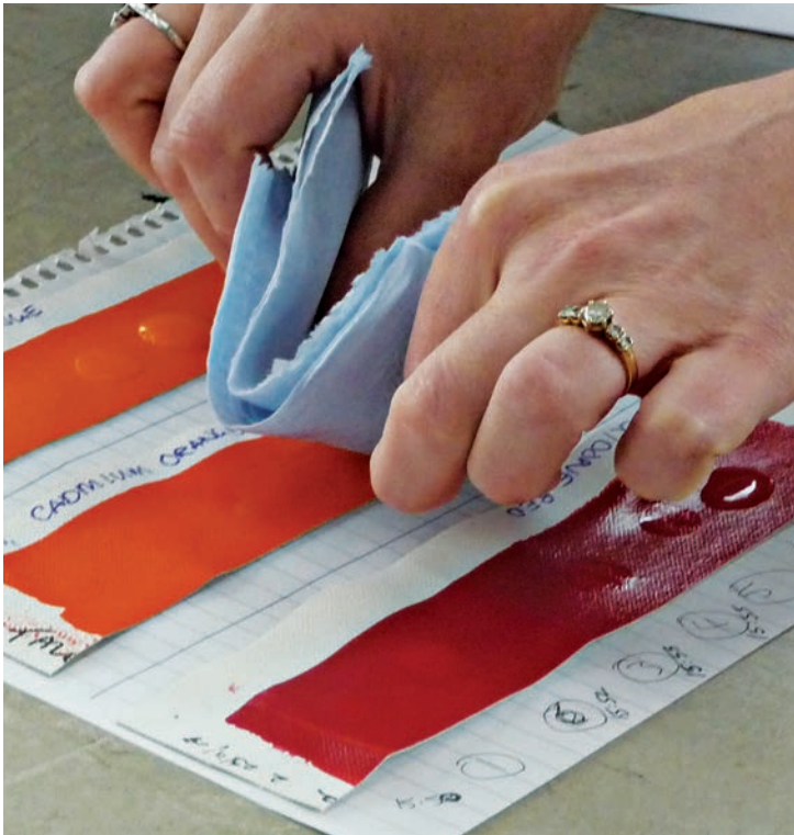
Above: A Cleaning of Acrylic Painted Surfaces (CAPS) workshop exercise , in which participants evaluate the relative swelling effect of different types of pH and conductivity-adjusted waters on unsoiled acrylic paint samples. Photo: © 2015 Tate. Right: The July 2016 CAPS workshop , organized by the GCI with the John and Mable Ringling Museum of Art in Sarasota, Florida. Instructor Bronwyn Ormsby overlooks the work of conservator Shauna Young. Photo: Tom Learner, GCI.
