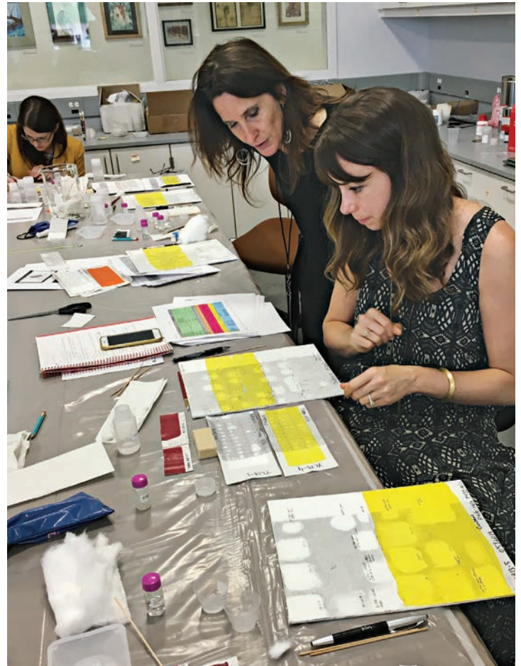
Above: A Cleaning of Acrylic Painted Surfaces (CAPS) workshop exercise , in which participants evaluate the relative swelling effect of different types of pH and conductivity-adjusted waters on unsoiled acrylic paint samples. Photo: © 2015 Tate. Right: The July 2016 CAPS workshop , organized by the GCI with the John and Mable Ringling Museum of Art in Sarasota, Florida. Instructor Bronwyn Ormsby overlooks the work of conservator Shauna Young. Photo: Tom Learner, GCI.
