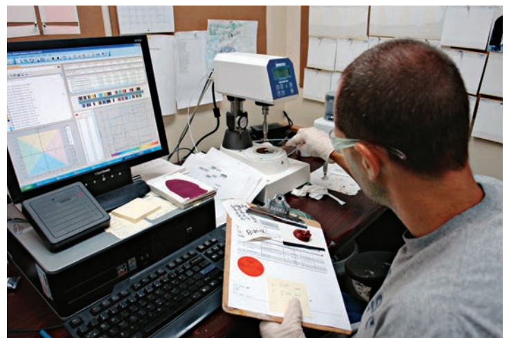
A technician measures the viscosity of oil paint on a cone-plate viscometer to assure consistency of product from batch to batch. Photo: Courtesy Golden Artist Colors, Inc.
