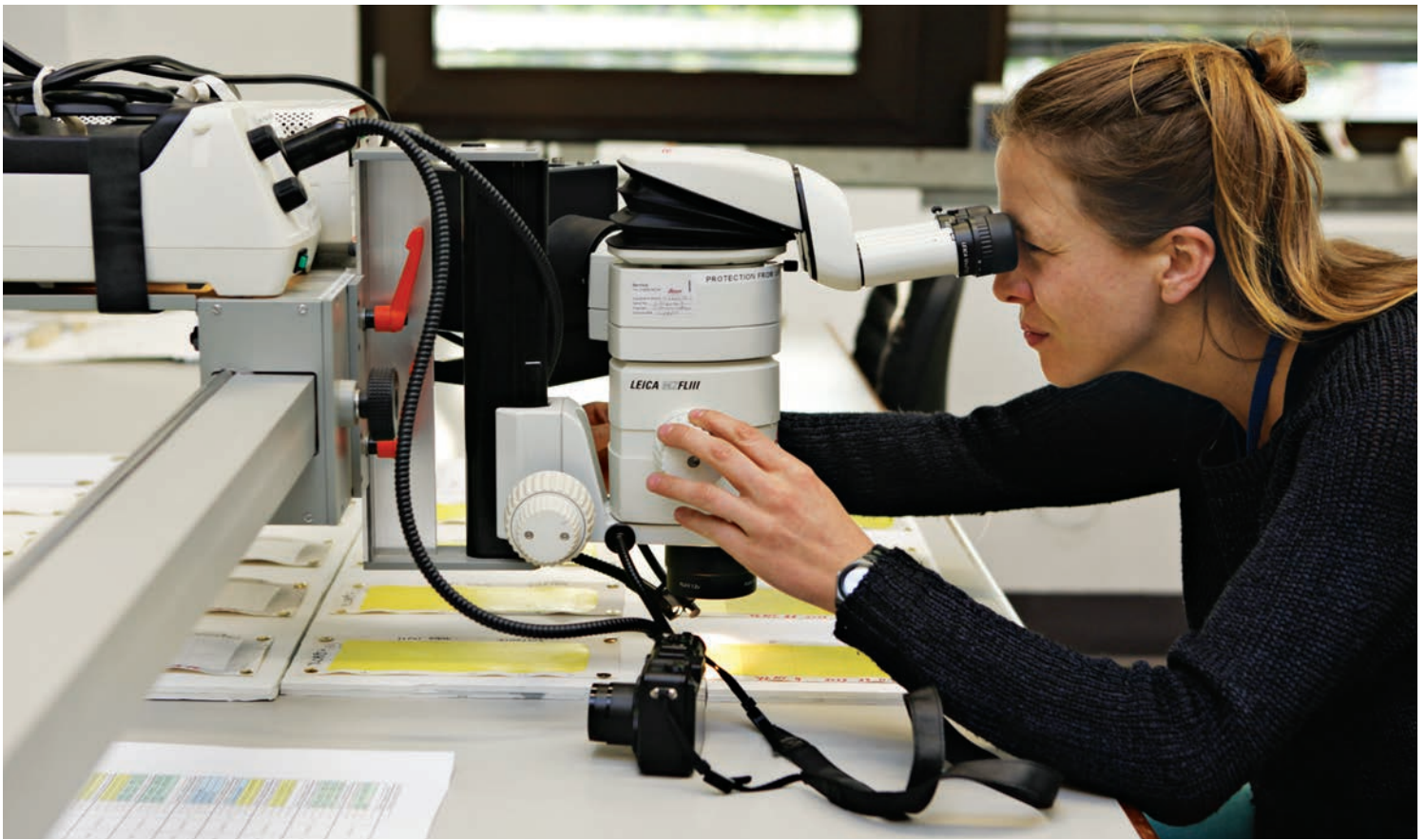
Josefina López using stereomicroscopy to examine the effects of surface cleaning materials on acrylic paint samples. Photo: © 2015 Tate.
