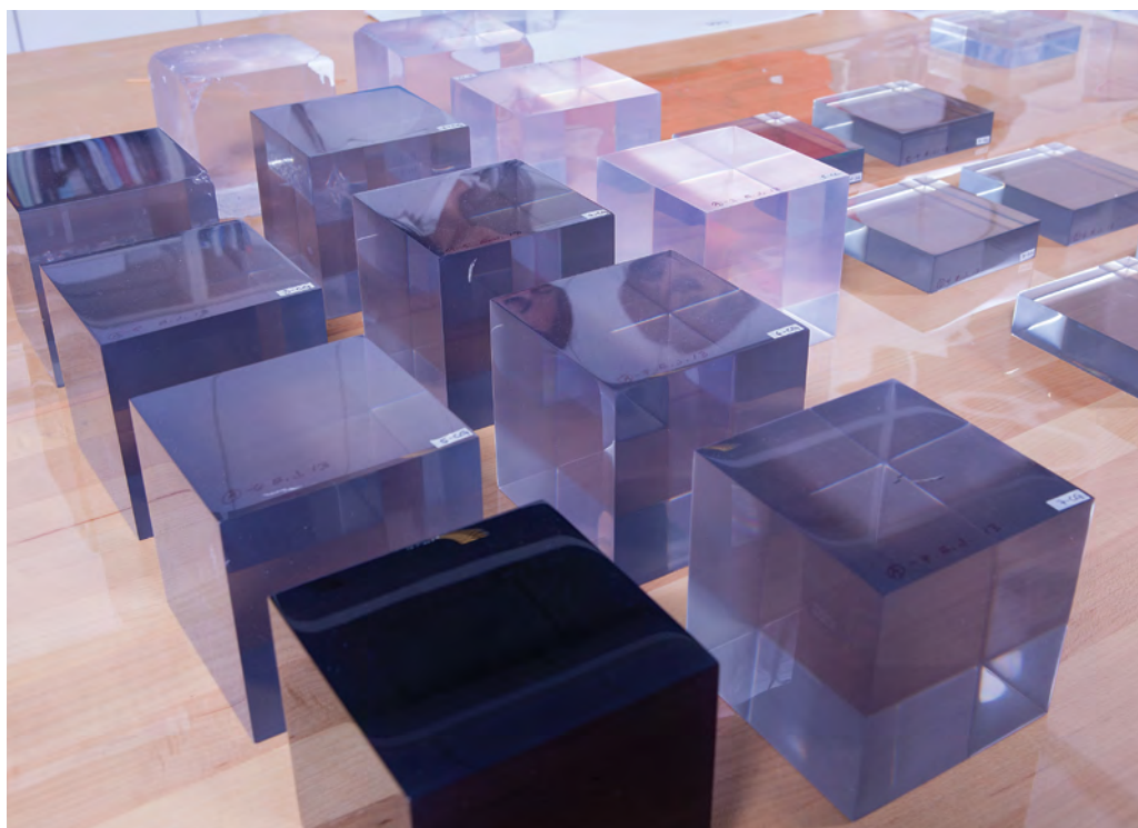
Polyester test samples being used in GCI research exploring minimally invasive techniques to repair plastic works of art. Photo: Anna Flavin, GCI.
