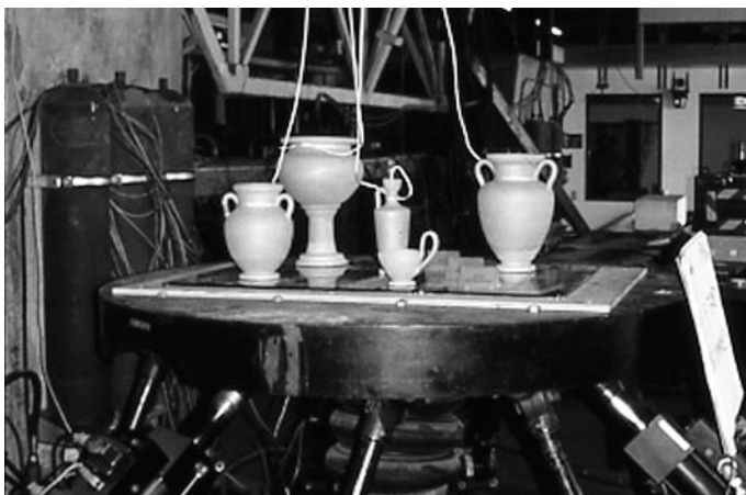
Ceramic replicas of ancient vases mounted in a variety of ways on a testing table that mimics seismic activity. Photo: Courtesy J. Paul Getty Museum.
