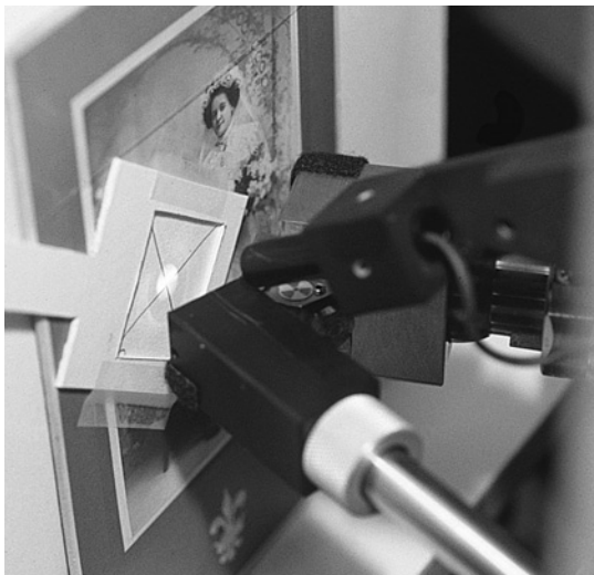
Quantitative X-ray fluorescence (XRF) analysis of photographs. XRF analysis—a nondestructive technique requiring neither sampling nor direct contact with the photograph—provides qualitative and quantitative information about inorganic elements in photographic material. Photo: Dusan Stulik.
