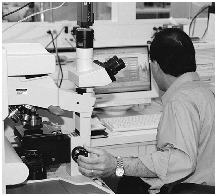
GCI assistant scientist Herant Khanjian conducting an analysis using Fourier transform infrared spectrometry (FTIR). FTIR provides information on organic components in a photograph without sampling or direct contact. The new GCI project will further develop a methodology of FTIR analysis of photographic material. Photo: Dusan Stulik.
