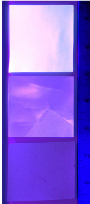
Unbrightened paper, unbrightened paper contaminated with optical brightener; optically brightened paper, photographed using near ultraviolet radiation.
