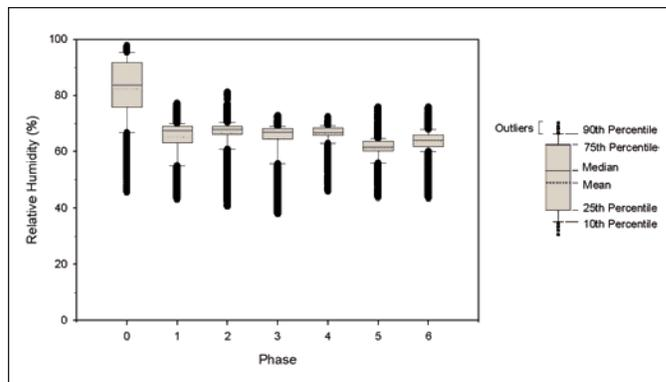
Fig. 5. Box plots showing basement relative humidity by phase.
