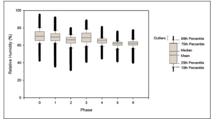
Fig. 7. Box plots showing attic relative humidity by phase.
