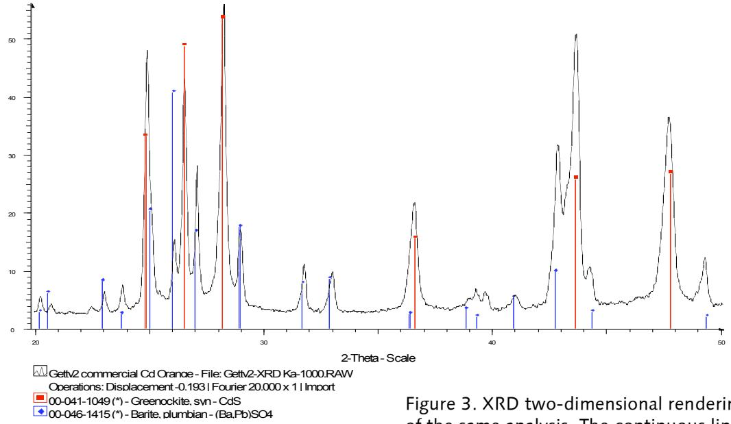
Figure 3. XRD two-dimensional rendering of the same analysis. The continuous lines are identified as cadmium sulfite and selenite ( $\text{CdS}/\text{CdSe}$  – in red), while the dotted lines are due to barite (barium sulfate – in blue), added as a filler.
