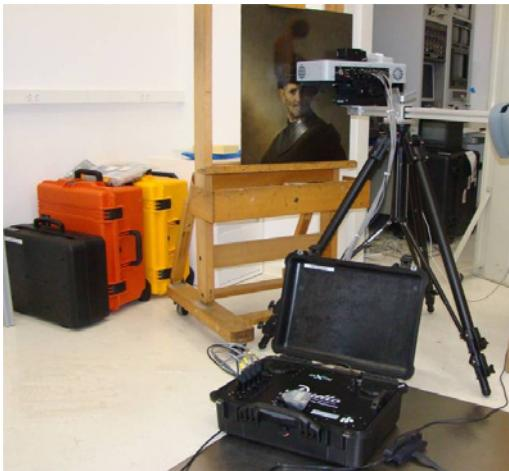
Figure 1. The head of the instrument is positioned in front of a painting and is supported by a sturdy tripod. On the front, there is a control unit. The whole system can be shipped in the three pelican cases seen in the back.
