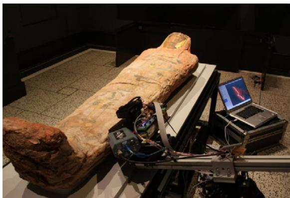
Figure 5. The XRD/XRF prototype, still to be fine-tuned, was used to analyze the pigments of the Red Shroud Mummy of the J. Paul Getty Museum's Antiquities 91.AP.6. Photo: G. Chiari.
