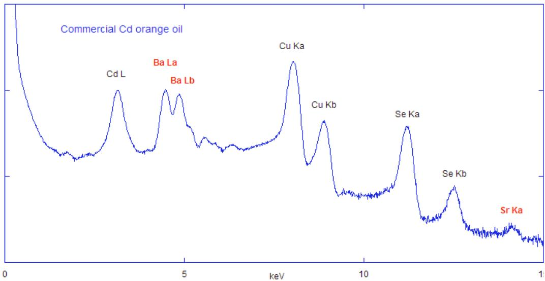
Figure 4. XRF pattern which shows cadmium, selenium and, unexpectedly, barium. The two lines of  $\text{CuK}\alpha$  and  $\text{CuK}\beta$  are due to the X-ray tube emission and are always present.
