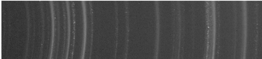
Figure 2. Image of the CCD detector. One can see the continuous diffraction lines, indicating that the crystals are very fine as randomly oriented. There are a few dotted lines, due to the presence of large crystals in a poorly crushed powder. The sample analyzed was a cadmium orange commercially manufactured color.
