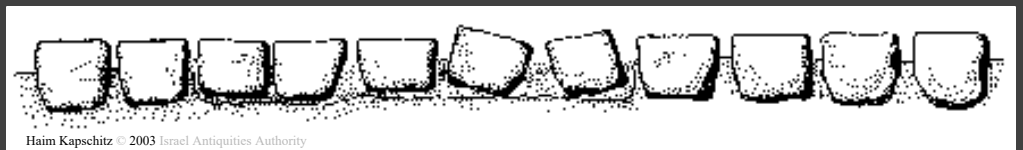
Tesserae detached from bedding layer with change of position (center)
