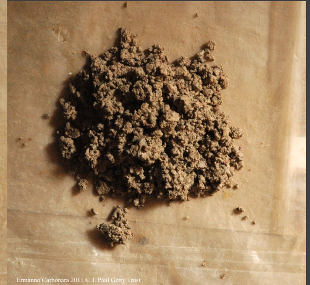
Mortar with too little water
