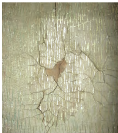
象身上起甲部分似乎已经用某种胶处理过，但是谁在什么时候执行这项工作却不清楚。 Area of flaking on the elephant that appears to have been treated with some kind of adhesive. It is unknown who carried out this work and when this treatment occurred.
