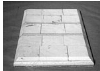
Figure 10 Balsa blocks trimmed and smoothed.
