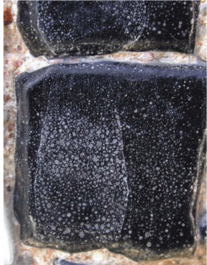
FIGURE 3 Coating problems: close-up view of blue tesserae with bubbles that formed underneath one of the tested (and rejected) coating systems.
