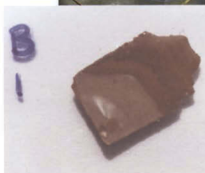
FIGURE 8 a, b Testing plate with coated original tesserae and artificial high-potassium glass (a). Delamination of epoxy coating after eight days of exposure in test chamber (b).
