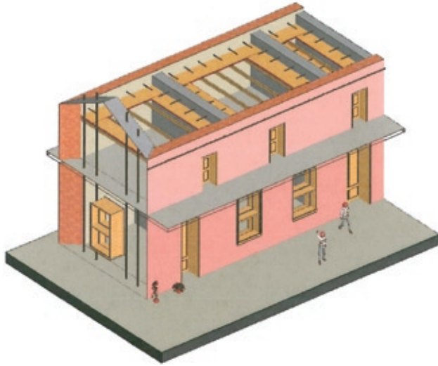
FIGURE 2 Selective use of full-height center core rods shown at the near gable-end wall, in the retrofit of the Castro-Breen Adobe. A partial plywood diaphragm with a horizontal exterior rod is used just below the roofline.
