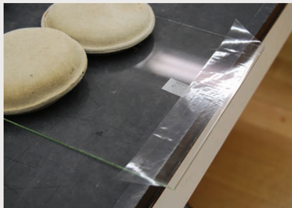
Figure 1b Step b. Apply packing tape strips to each side of the glazing. Fold each packing tape strip back onto the glazing and temporarily hold it with tape. Photo: M. Alan Miller.
