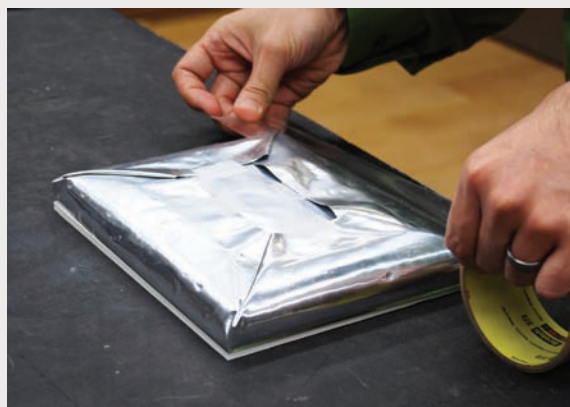
Figure 1f Step f. Remove the Marvel Seal envelope package from the frame and carefully tape-seal all joints. This package can now be secured into the frame. Photo: M. Alan Miller.
