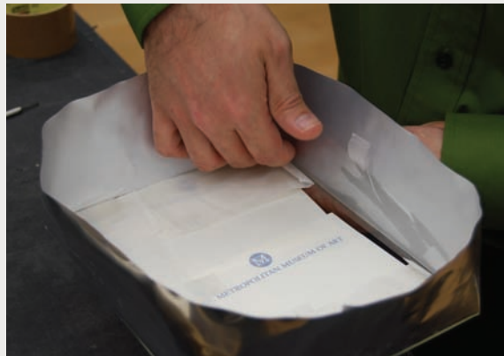
Figure 1d Step d. Carefully bring up each packing tape strip (now on the inside) and adhere it to the inside of the perimeter strip. Photo: M. Alan Miller.
