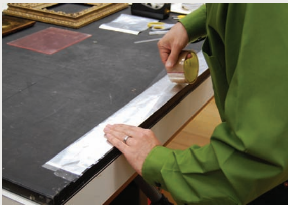
Figure 1a Step a. Cut a perimeter strip of Marvel Seal long enough to wrap around the glazing. Apply a continuous piece of clear packing tape along one edge of this strip, leaving about 7 mm (0.3 in.) hanging off the edge (this measurement corresponds to the thickness of the glazing, plus extra to adhere to the front). Photo: M. Alan Miller.
