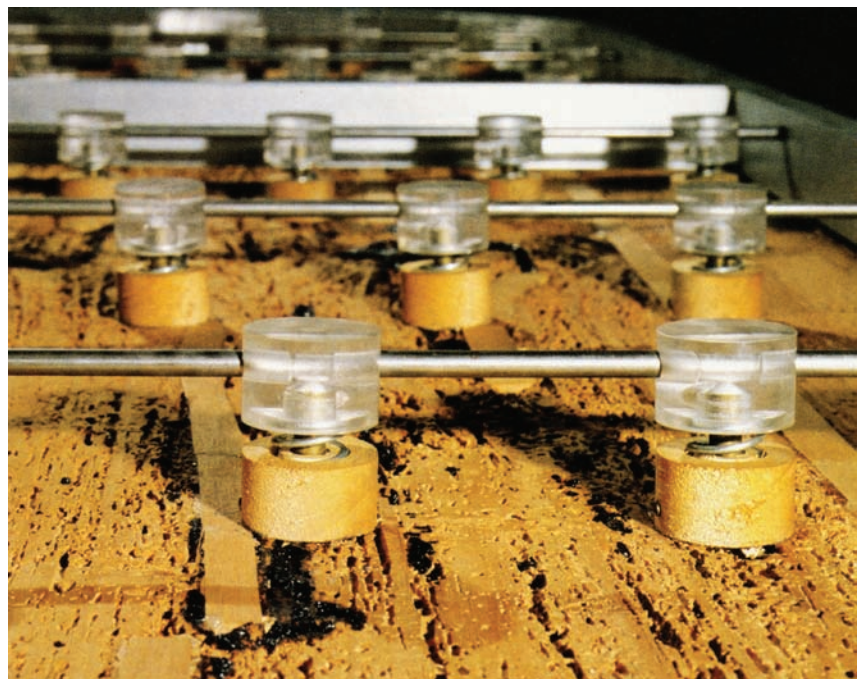
Figure 1 Basile-Mancinelli-Trevisani spring mechanism developed at ICR around 1979–80. Photo: Courtesy of Eugenio Mancinelli.
