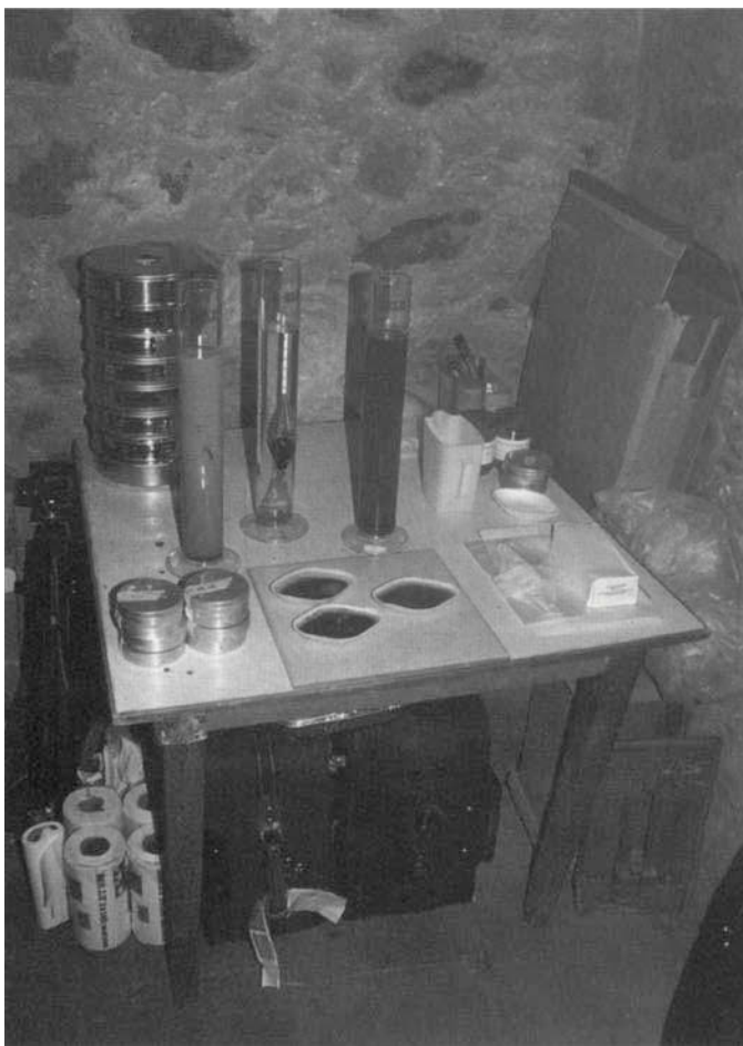
FIGURE 5 Temporary earthen-materials analysis laboratory set up in the narthex of the church. Photo courtesy of the Courtauld Institute of Art, Conservation of Wall Painting Department, 2002.
