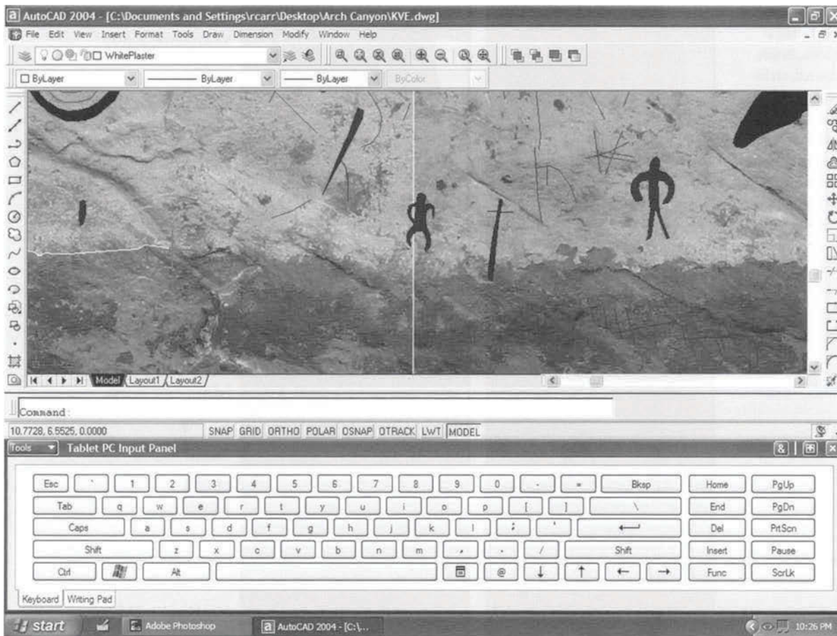
FIGURE 5 Graphics tablet PC screen from the laptop computer used to digitize documentation of surface finishes while working in the field. Graffiti and historic iconography are outlined using AutoCAD 2004. Courtesy of ASCP Digital Archives, Mesa Verde National Park. Documentation and graphics by Rebecca Carr.
