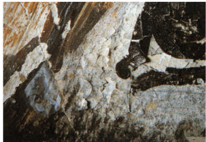
FIGURE 6 Census of Cattle (EA37976): 1.75x magnification of paint lifted by carnauba wax. Photo: Eric Miller.
