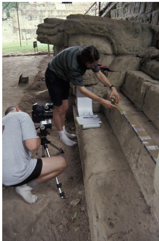
Figure 51 Photarc Surveys Ltd. consultants taking stereophotographs of block 2 using a medium-format camera.
