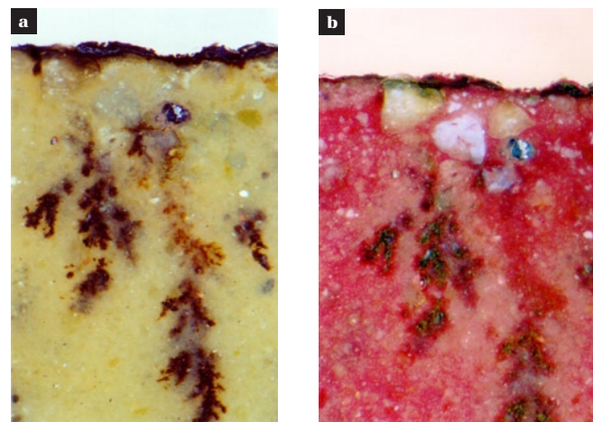
Figures 80a and b Cross section (a) and cross section stained with PAS (b) (x114), showing the deep fungal penetration in the quarry samples.
