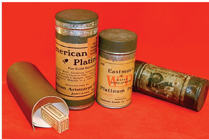
Figure 3 Three different kinds of commercial platinotype paper in their original metal tubes, shown with a capsule of calcium chloride desiccant that was used to extend the shelf life of platinotype paper.
