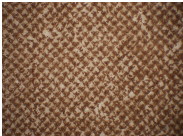
Figure 15a Detail of the print in fig. 14 (40× magnification), showing a typical rotogravure pattern.
