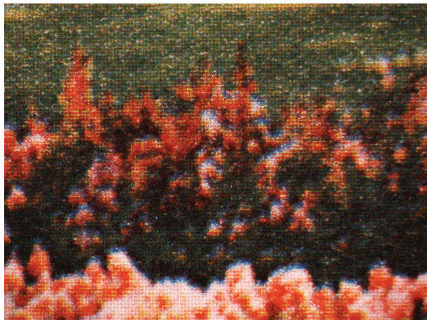
Figure 24a Detail of the print in fig. 23 (10× magnification), showing a three-color rotogravure pattern.
