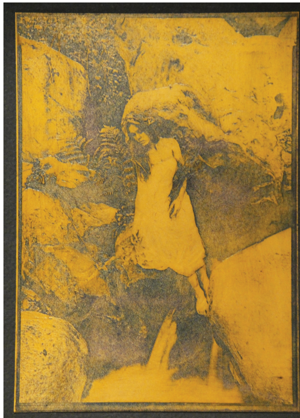
Figure 35 Fully processed and inked photopolymer gravure plate.
