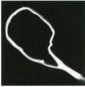
FIGURE 9. CT slice of Roman bronze bull, first century B.C.E. to first century C.E., showing extent and specific depth of plaster restorations.
