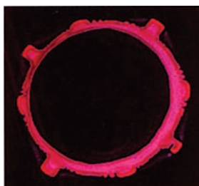
FIGURE 2. CT slice of Chinese Shang Dynasty gu wine beaker. Section taken through circular base shows uneven wall thickness due to misalignment of core with respect to mold.
