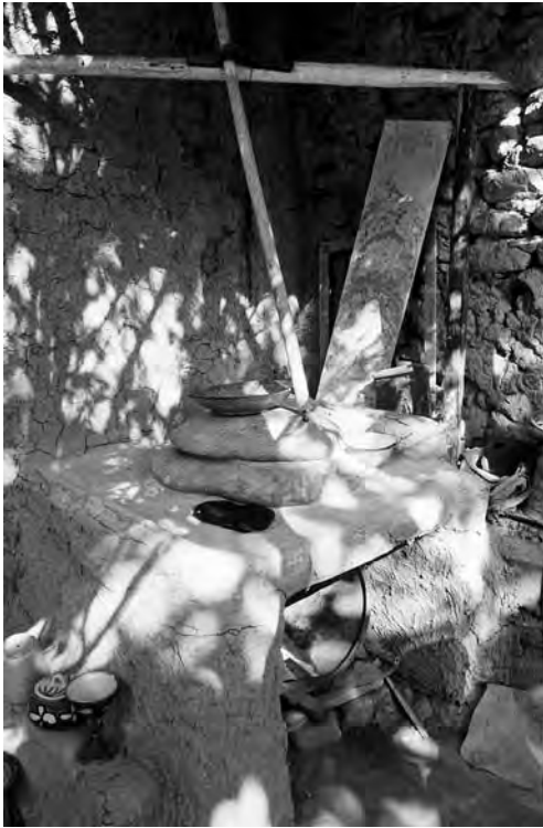
FIGURE 7 Hand-operated quern for milling ishkor ash, with a bowl of ash for one milling operation on the top in the courtyard of the Marajapov family.
