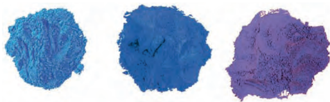
FIGURE 2 Left: Egyptian blue ( \text{CaCuSi}_4\text{O}_{10} ); middle: Chinese purple ( \text{BaCuSi}_2\text{O}_6 ); right: Chinese blue ( \text{BaCuSi}_4\text{O}_{10} ).
