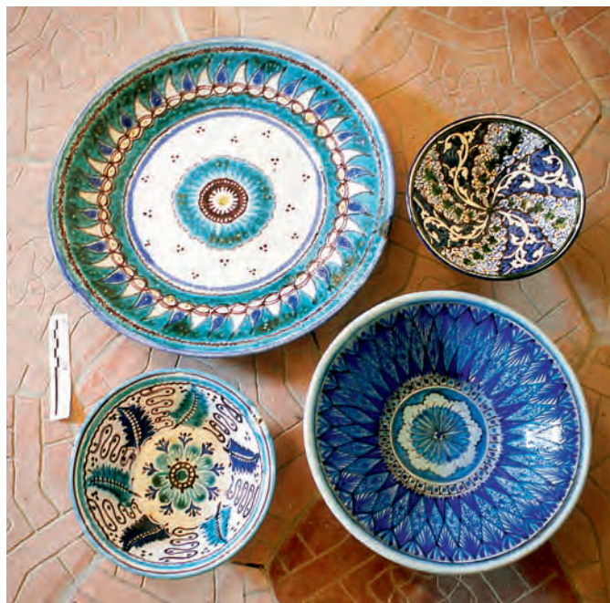
FIGURE 10 Four bowls by Ibrahim Kamillov, each showing a variation on the ishkor technique. Note the difference in gloss as shown in the specular reflectivity. The right side shows two bowls in traditional ishkor technique: the upper one with no lead oxide addition and the lower one with low lead. The left side shows two innovative bowls: the upper one with high barium oxide and the lower one with very high lead oxide content.
