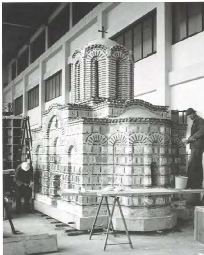
The scale model of the Church of St. Nikita, constructed to test seismic stabilization techniques. Photo courtesy of the Institute of Earthquake Engineering and Engineering Seismology.
