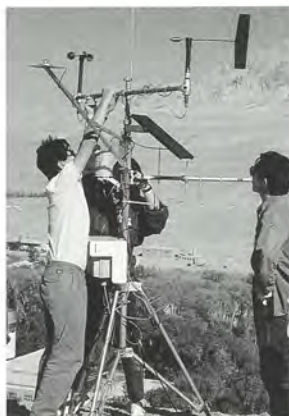
Above left: Shin Maekawa of the Institute installing the environmental monitoring station at the Mogao Grottoes, assisted by Chinese project team members. Photo: R. Tseng.
