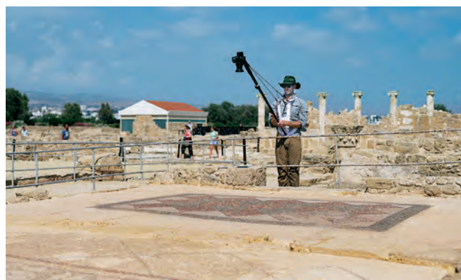
Photogrammetric capture being conducted on exterior mosaics at Nea Paphos by GCI staff member Thomas McClintock. Photo: Silvio Augusto Rusmigo, for the GCI.
