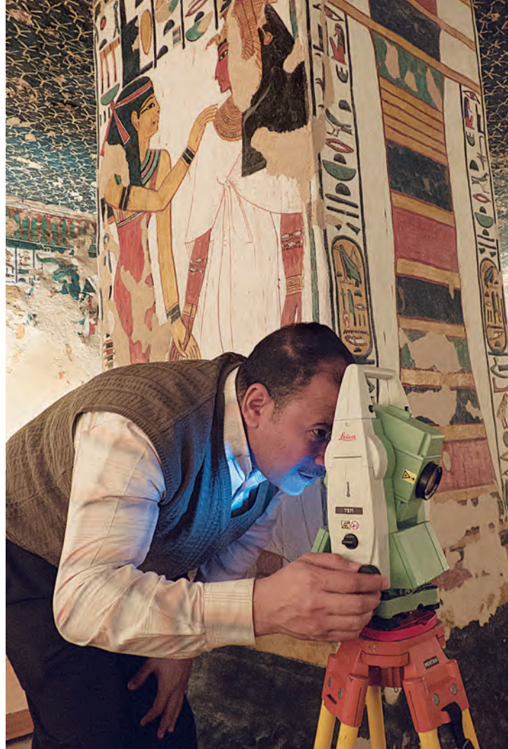
A total station collecting spatial data in the tomb of Nefertari in Egypt. A total station is an electronic/optical instrument used in surveying and just one of the many tools available to create data. Photo: Carleton Immersive Media Studio, ©The J. Paul Getty Trust.
