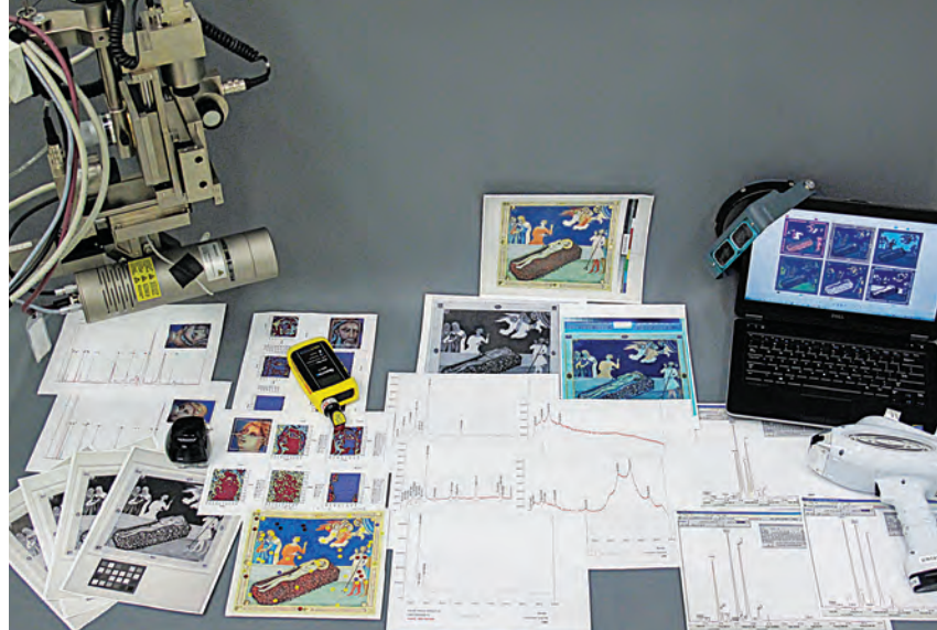
Examples of scientific data collected on a museum object and some of the equipment used to collect that data. Seen here are various images, XRF spectra and element distribution maps, Raman spectra, and a data visualization of The Martyrdom of Saint Lawrence , Pacino di Bonaguida, about 1340. Tempera and gold leaf, Leaf: 19 × 20.8 cm (7 1/2 × 8 3/16 in.). The J. Paul Getty Museum, Los Angeles, Ms. 80b, verso, 2006.13.verso. Photo: Catherine Patterson, GCI, ©The J. Paul Getty Trust.
